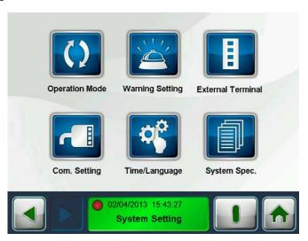
To enter various function settings under system settings, the screen will prompt for password entry, the default password is: "20120123". The various functions can only be displayed or set after successful password entry (as shown in the figure below).
