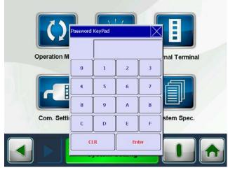
Note 1: The default password is: "20120123". This password can only access settings for basic functions. After entering the password, all functions can be accessed freely. If the system is inactive for more than 10
