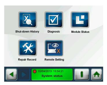
1) Shut-down History: This function records failures during operation; warnings are not included. Records 200 sets of occurrence time (hh:mm:ss), date (mm:dd:yyyy) and details of the failure.
