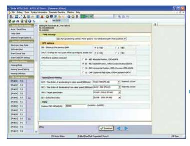
Easy-to-use editing interface is designed for new and enhanced PR control mode. Homing, point-to-point and other motion control functions for multi-axis positioning control are easily achieved.
