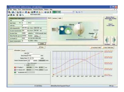
User-friendly E-CAM editing interface is provided for designing E-CAM outlines and curves freely. In addition, quick settings for flying shear and rotary cut applications are offered.
