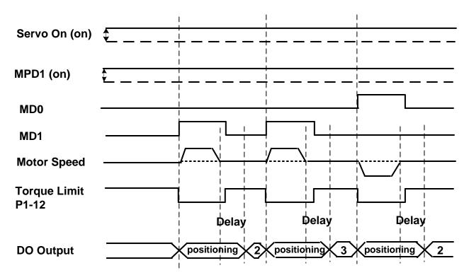
Figure (3.19) Timing diagram for manual index control
