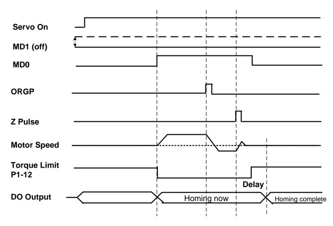
Figure (3.15) Timing diagram for homing process
