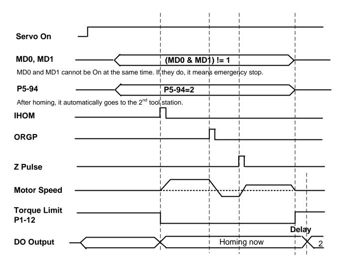
Figure (3.16) Timing diagram of moving to next tool station after homing
