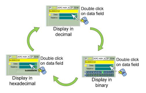
Figure (3.22) Switch the display format of scope signal
