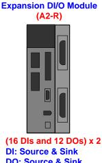
**DI: Source & Sink DO: Source & Sink** 0.4KW ~ 3KW
