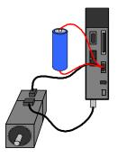
Absolute system (A2 or A2R) (motor with optical system)
