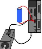
Absolute system (A2R) (Motor with optical encoder)
