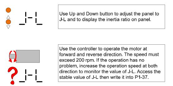
Figure (3.25) Use panel to read inertia ratio
