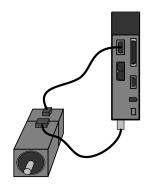
Incremental system(A2R) (Motor with magnetic encoder)
