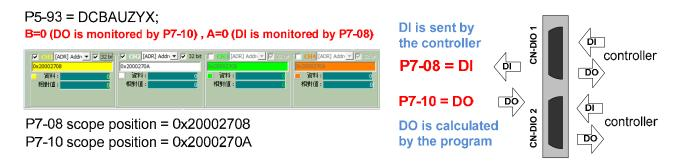
Figure (3.20) Monitor the DI/O status on extension module
