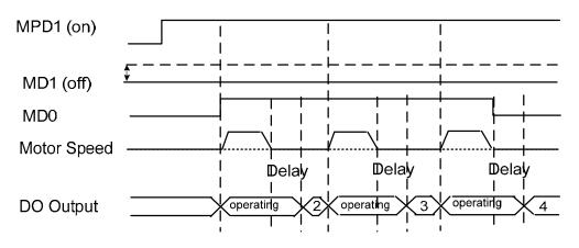
Figure (3.5) Time sequence when stopping at every station
