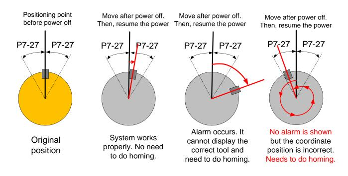
Figure (3.9) Allowable range for magnetic encoder
