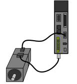
Incremental system (A2 or A2R) (motor with optical encoder)
