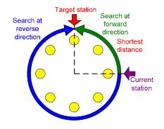
Figure (3.7) Target station searching method
