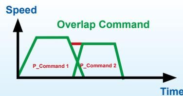
The speed command is executed after the delay time or during the deceleration period.
