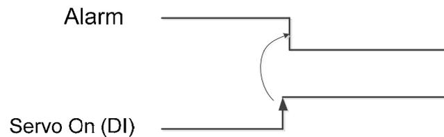
Figure (3.11) Method to clear the alarm
