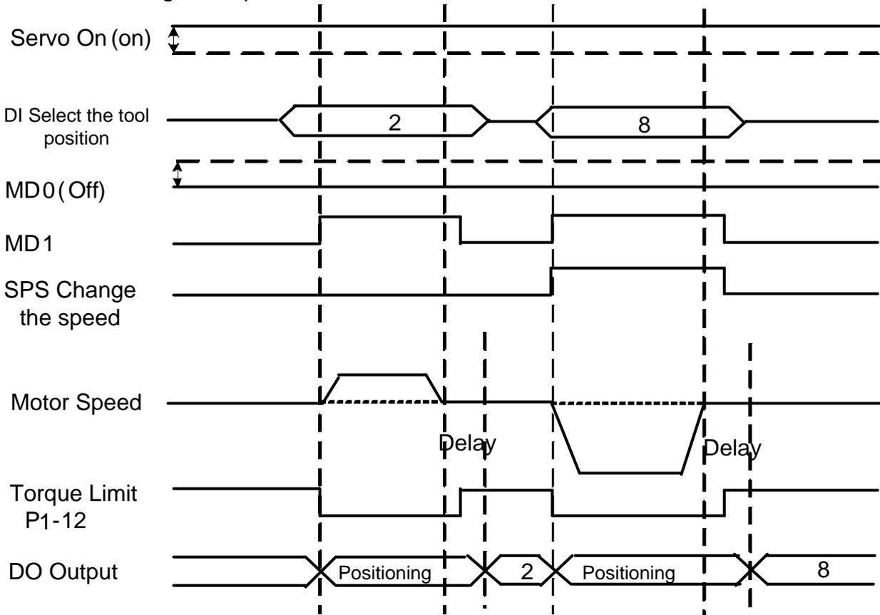
Figure (3.18) Timing diagram of auto operation with speed switching
