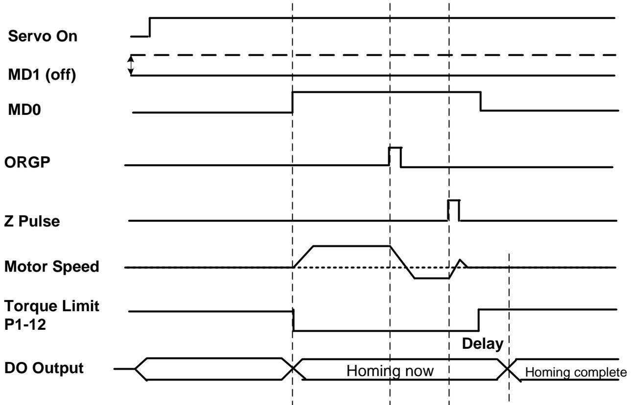
Figure (3.15) Timing diagram for homing process
