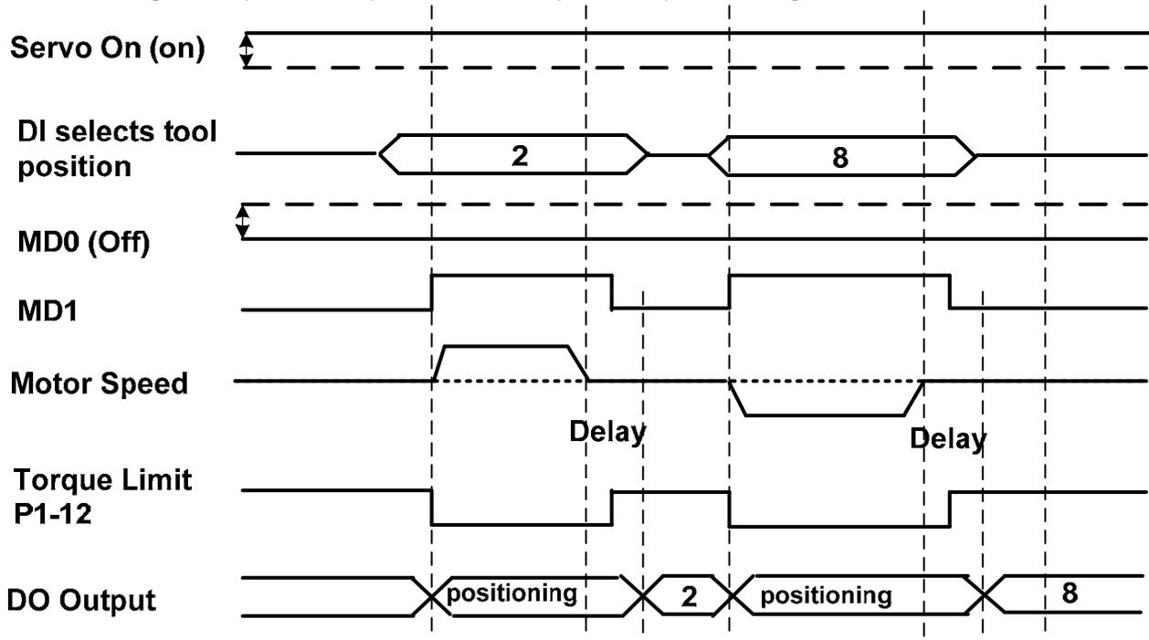
Figure (3.17) Timing diagram of auto operation with one speed setting
