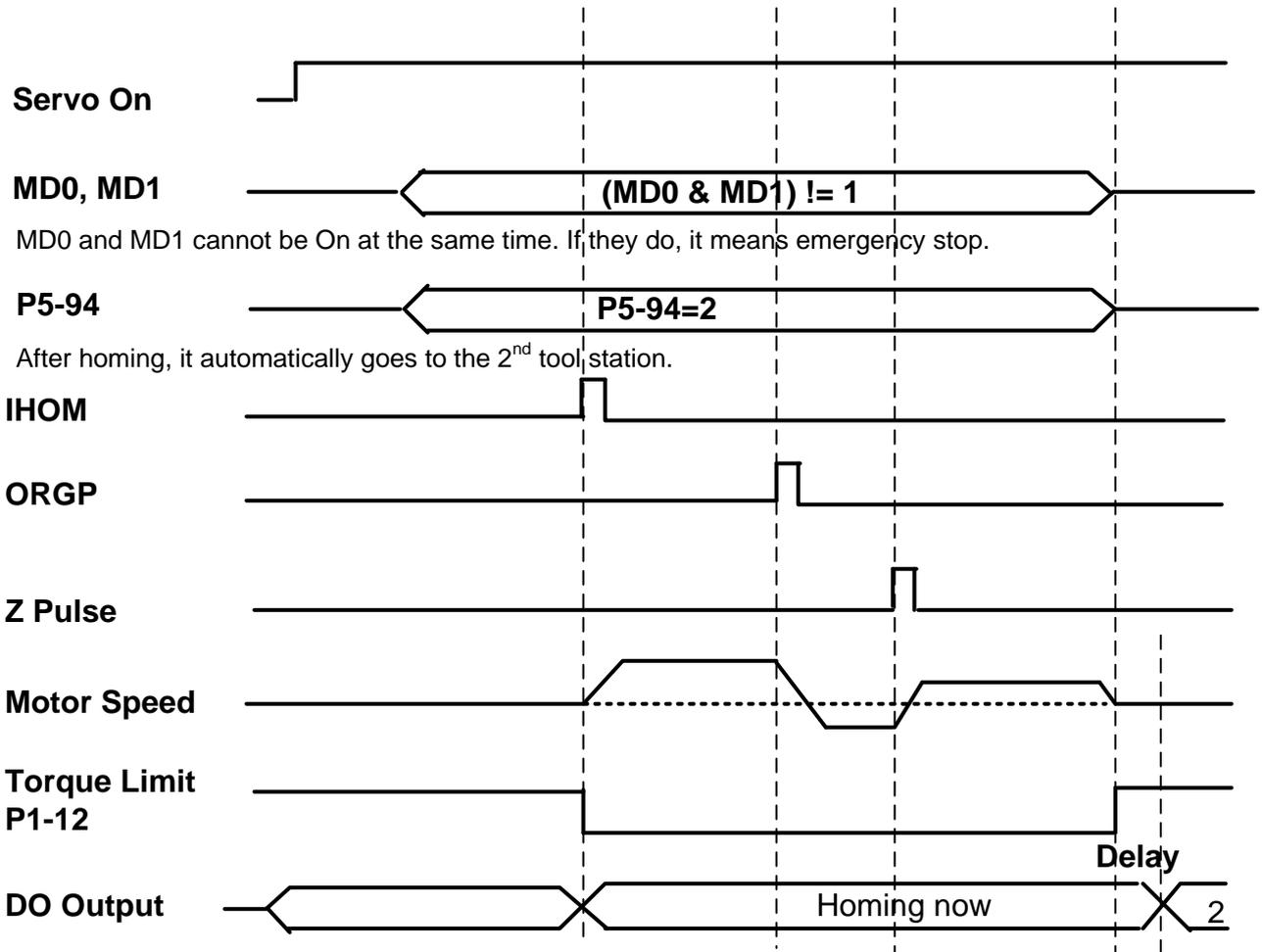
Figure (3.16) Timing diagram of moving to next tool station after homing
