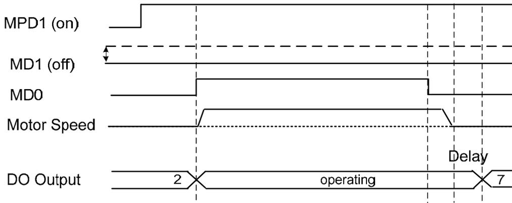
Figure (3.6) Time sequence when stopping at the nearest station
