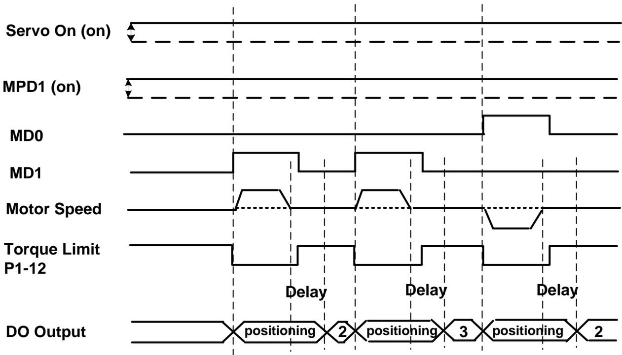
Figure (3.19) Timing diagram for manual index control
