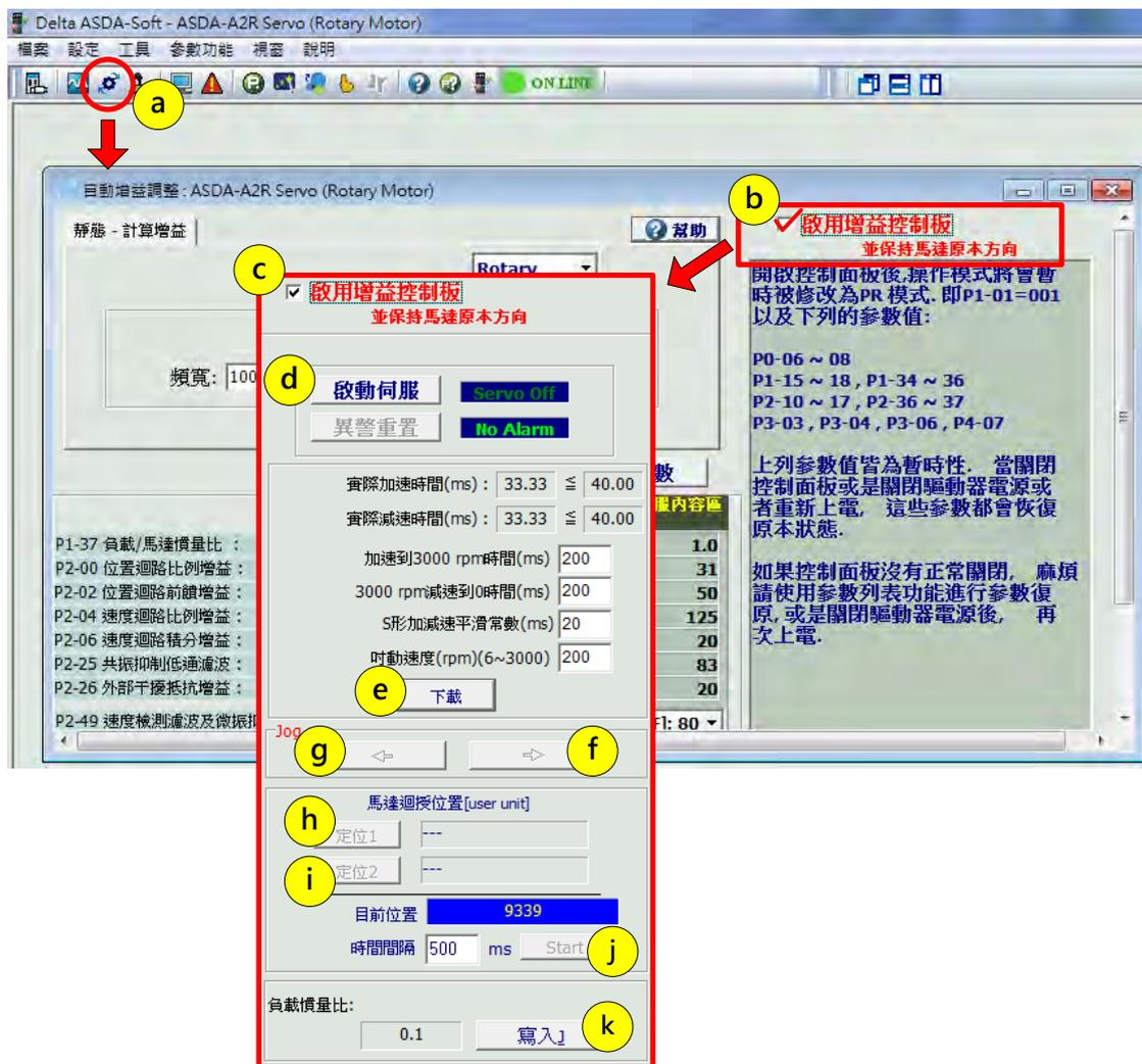
Figure (3.23) Inertia estimation
