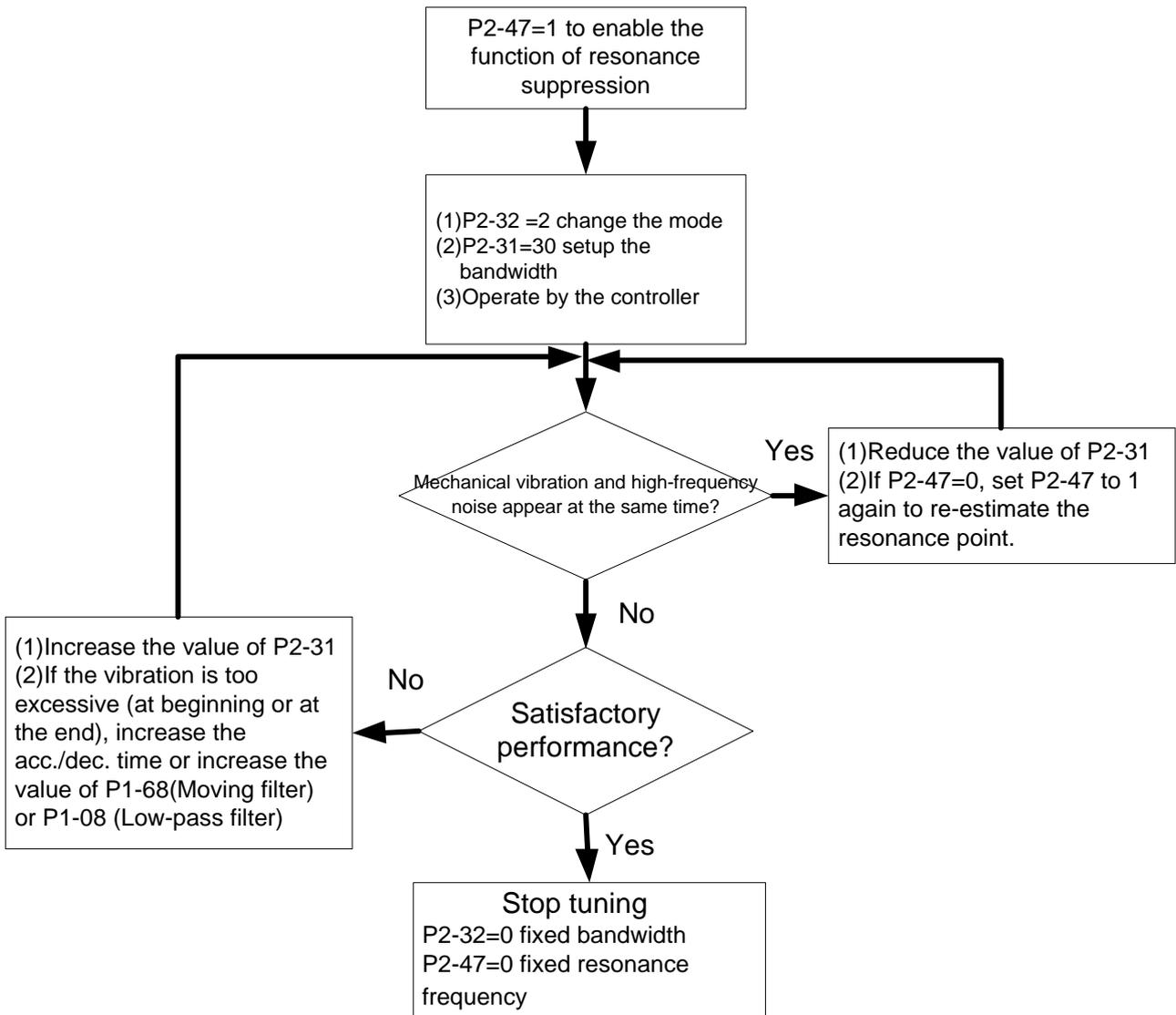
Figure (3.26) Use panel to tune the system
