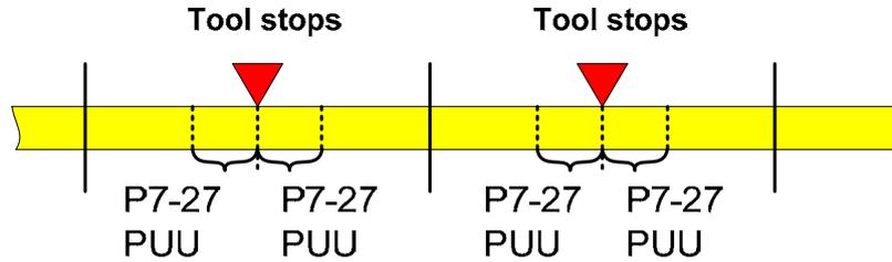
Figure (3.8) Tool position range confirm
