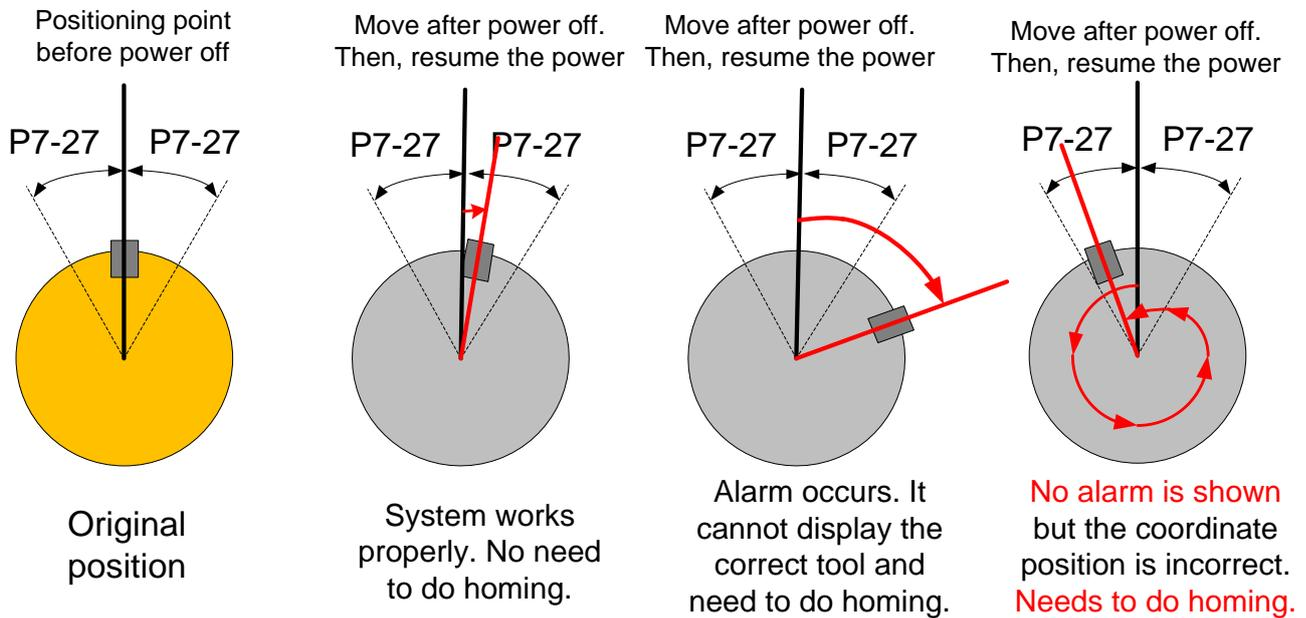
Figure (3.9) Allowable range for magnetic encoder
