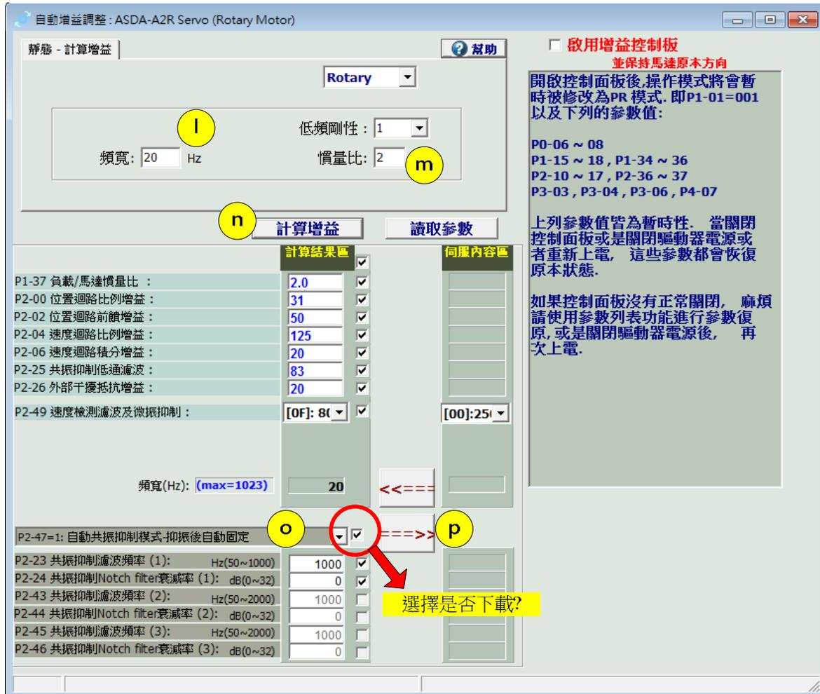
Figure (3.24) Compute and Download the Gain
