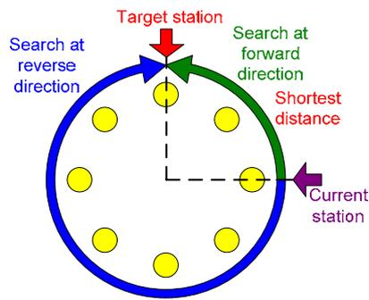
Figure (3.7) Target station searching method
