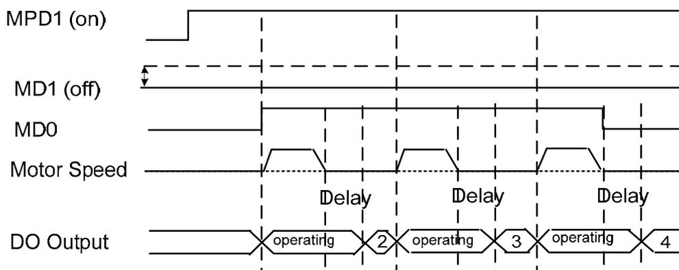
Figure (3.5) Time sequence when stopping at every station
