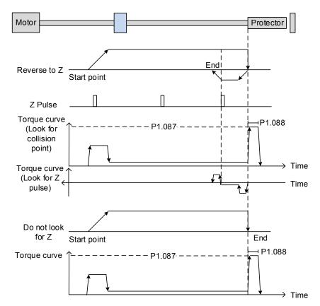
In the figure above that uses looking for the Z pulse, the motor runs at the high speed (first speed setting). Then the servo outputs a greater current to resist the external force once the motor touches the collision protector. When the motor torque reaches the set limit (P1.087) and the output duration is longer than the time setting (P1.088), the motor runs in
