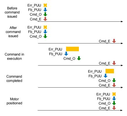
Figure 7.1.2.1 Timing diagram for PR mode monitoring variables
