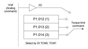
When using the Torque Limit function, you can set this parameter to 1 to limit the torque permanently without occupying a DI setting. Alternatively, you can enable or disable the limit function through DI.TRQLM, which is more flexible, but the setting then occupies a DI setting. You can enable the Torque Limit function by either P1.002 or DI.
