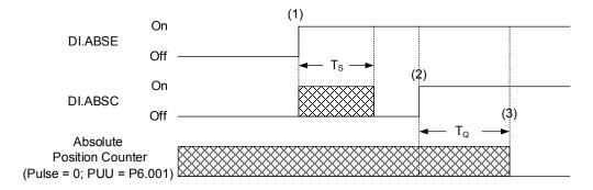
Figure 10.3.4.1 Timing diagram for initializing the absolute coordinate system with DI/DO The following table describes the  $T_S$  and  $T_Q$  delay time after triggering DI.ABSE and DI. ABSC.
