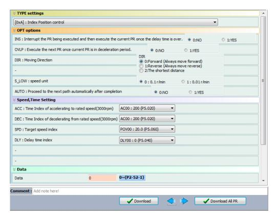
Figure 7.1.3.14 PR mode Index Position screen in ASDA-Soft
