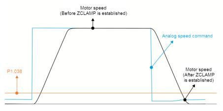
1: command source is the internal register. ZCLAMP function uses the register Speed command with acceleration / deceleration to determine if this function should be enabled. When ZCLAMP conditions are met, the motor speed is set to 0 rpm.
