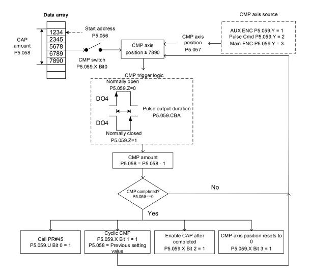
Figure 7.2.3.1 Flow chart for the high-speed position Compare function
