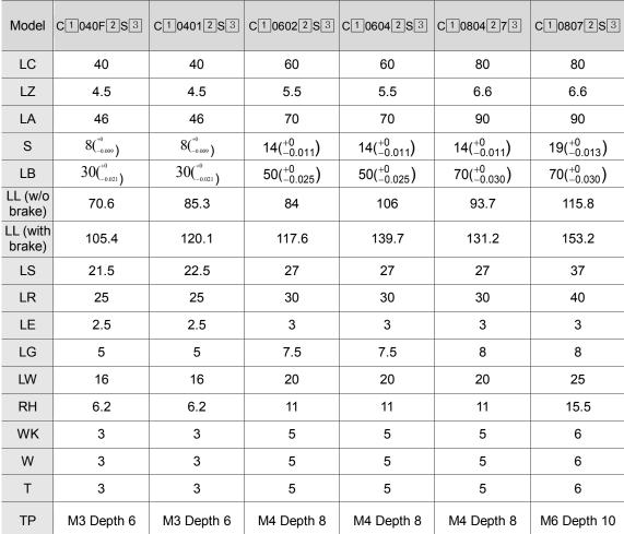
Note:  $\boxdot$  in motor model name represents the encoder type;  $\boxdot$  represents the shaft type and oil seal;  $\boxdot$  represents a special code.
