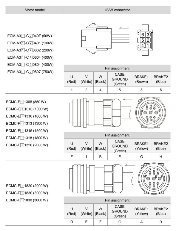
Wire selection: please use a 600 V PVC cable. If it is longer than 30 meters, refer to the voltage drop (wire impedance) to select the cable size. See section 3.1.6 for more information.
