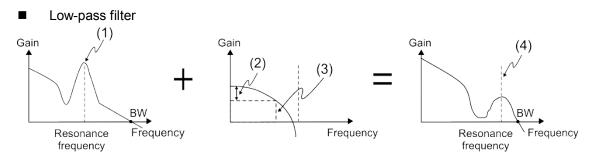
(1) Point of resonance (2) Attenuation rate (-3 dB)
