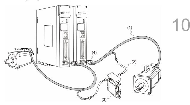
(1) Encoder cable; (2) Battery box cable AW; (3) Double battery box (absolute type); (4) CN2 connector
