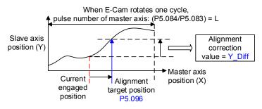
\*P5.093.UZ is able to limit the maximum correction rate. The alignment target position ★ will be different from P5.096.
