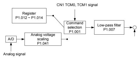
Control in the upper path is from the register while the in lower path it is from the external analog voltage. You select the command according to the status of TCM0, TCM1, and P1.001 (T or Tz). You can adjust the torque with the analog voltage scaling (P1.041) and you can smooth the response with the low-pass filter (P1.007).
