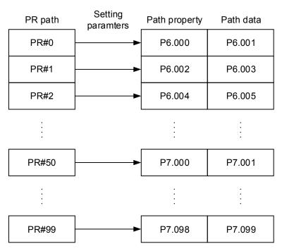
Figure 7.1.1 Setting parameters for each PR path
