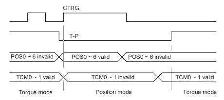
Figure 6.5.3.1 Torque / Position dual mode
