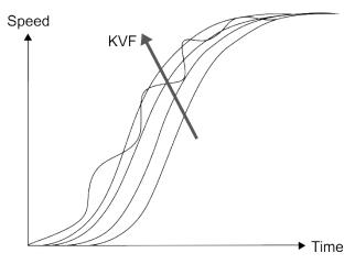
The closer the KVF value is to 1, the more complete the forward compensation. The following error becomes very small. But a KVF value that is set too high also causes vibration.
