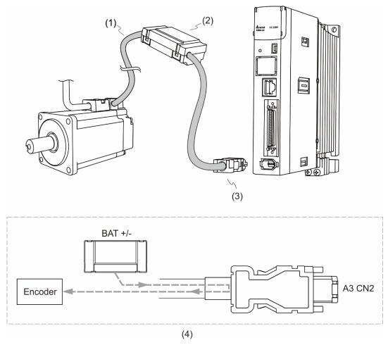
(1) Encoder cable; (2) Single battery box (absolute type); (3) CN2 connector; (4) Battery box wiring Pin assignment of CN2:
