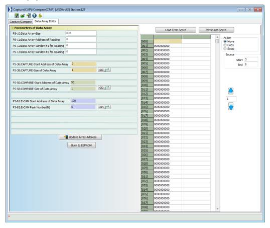
Figure 7.2.1.1 Data Array screen in ASDA-Soft
