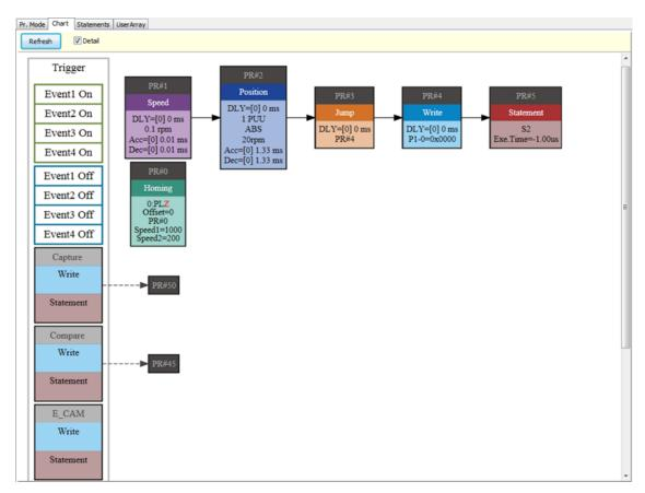
Figure 7.1.3 PR diagram display in ASDA-Soft
