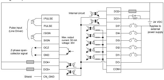
Wiring for CN1 quick connector and installation:
