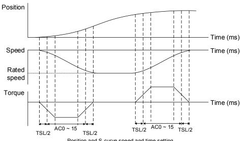
Position and S-curve speed and time setting (Deceleration for position command)
