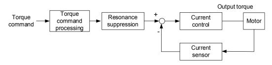
You use the Torque Command unit to specify the Torque command source (mentioned in Section 6.4.1), including the scaling of the analog voltage (P1.041) and the S-curve setting. The current control unit manages the gain parameters for the servo drive and calculates the current for servo motor in real-time; you can only set this by commands.
