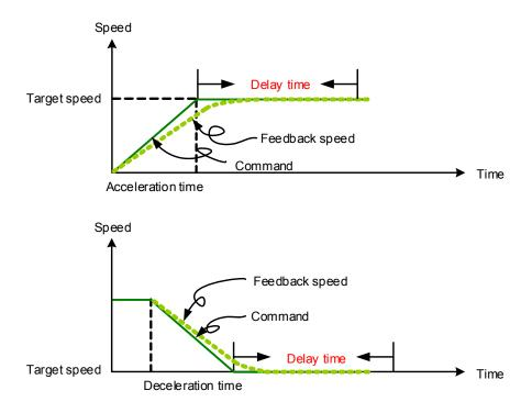
Figure 7.1.3.5 Parameters for PR mode speed control
