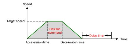
Figure 7.1.3.7 Parameters for PR mode position setting
