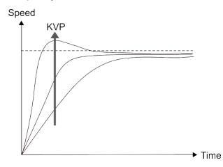
The higher the KVP value, the larger the bandwidth. The time of the speed increase will also be shorter. However, if the value is set too high, the phase margin is too small. The effect is not as good as KVI for the steady-state error but is better for the effect on following.
