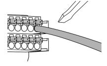
(4) Withdraw the screwdriver to complete the wiring.
