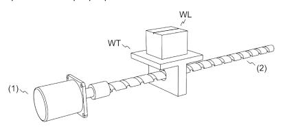
(1) Motor (2) Ball screw pitch: 3 mm (equals 3000 μm) WL: Workpiece; WT: platform
