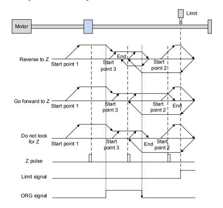
See the above example of looking for the Z pulse. If ORG signal is un-triggered at the start point (low, Start point 1), the servo motor runs at high speed (first speed setting) until reaching the rising edge of the ORG signal. Then it decelerates and switches to low speed until the ORG signal is off (low). Next, it reverses to look for the Z pulse and decelerates to a stop once it finds the Z pulse, completing the homing.
