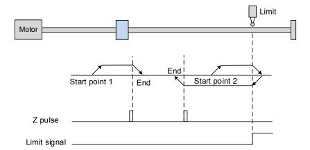
4. Referencing the falling-edge of the ORG signal. This method uses the falling-edge signal of the home sensor as the reference origin. You can choose whether or not to use Z pulse as the reference origin after the ORG signal is detected.
