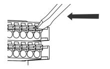
(2) Use a flathead screwdriver to press the spring down to open the pin.
