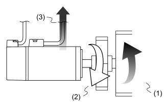
(1) Direction of motion of the object; (2) Force direction of the motor; (3) Regenerative power
