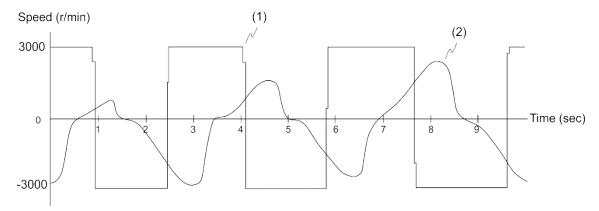
(1) Analog Speed command (2) Motor torque
