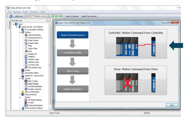
Suggestions: you should set the motor to operate at least one cycle in both forward and backward directions. It should reach the positions (in both forward and backward directions) in 1000 ms or less with the running speed not less than 500 rpm.
