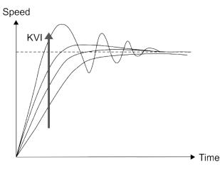
The higher the KVI value, the larger the low frequency gain. It shortens the time for the steady-state error to reduce to zero. However, it does not significantly reduce the following error.
