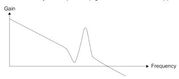
When the value of P2.025 is increased from 0, BW becomes smaller. Although it solves the problem of the resonance frequency, the response bandwidth and phase margin are reduced. Also, the system becomes unstable.
