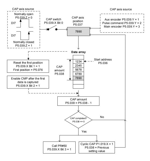
Figure 7.2.2.1 Flow chart for high-speed position capturing
