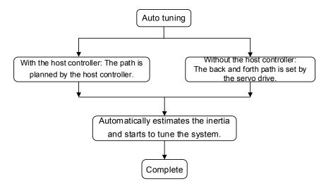
Note: when the running distance is configured by the host controller, make sure the delay time is added to the operation time. Otherwise, AL08C occurs and the servo drive cannot complete auto tuning.
