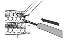
(3) Insert the stripped wire into the pin.
