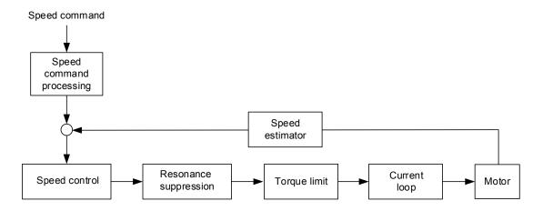
The Speed Command processing unit selects the command source (see Section 6.3.1), including the scaling parameter (P1.040) for rotation speed and S-curve parameter for smoothing the speed. The Speed Control unit manages the gain parameters for the servo drive and calculates the current command for servo motor in real-time. The Resonance Suppression unit suppresses the resonance of the machine.
