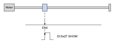
6. Referencing the torque limit. This method uses the motor's stop position as the origin by referring to: the limit on the mechanism, the torque level setting (P1.087), and the retaining time (P1.088). You can also choose whether to use the Z pulse as the origin.
