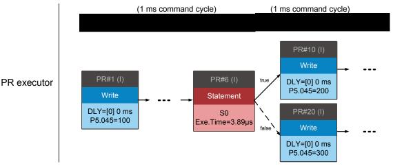
Figure 7.1.6.12 Multiple commands with arithmetic operations
