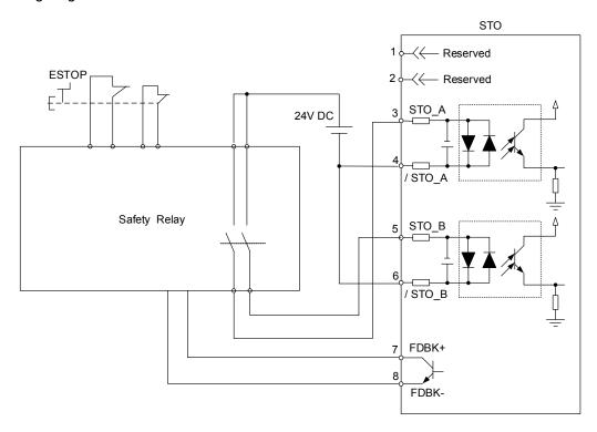
If you are not using the STO function, you can short-circuit the connector or plug in the connector that has been wired (provided with the servo drive).
