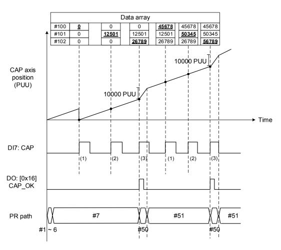
Figure 7.2.2.4 Application example for high-speed capturing function
