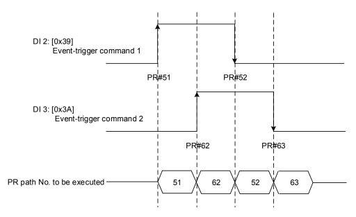
Figure 7.1.5.3 Example of Event triggering timing diagram
