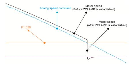
0: command source is the internal register. ZCLAMP function uses the register Speed command with acceleration / deceleration to determine if this function should be enabled. The motor is clamped at the position where ZCLAMP conditions are met.
