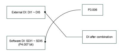
Read parameters: shows the DI status after combining external DI and software DI.
