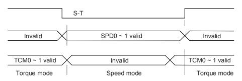
Figure 6.5.2.1 Speed / Torque dual mode
