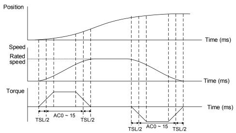
Position and S-curve speed and time setting (Acceleration for position command)
