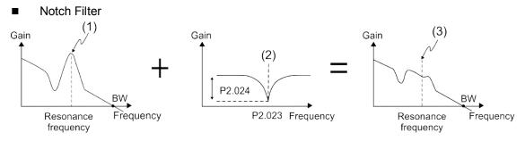
(1) Point of resonance (2) Notch filter (3) Point of resonance suppressed by the Notch filter
