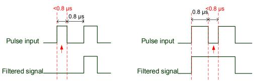
If this first pulse width is shorter than 0.8  $\mu s,$  it may be filtered, and thus two input pulses will be regarded as one pulse. If this pulse width is shorter than 0.2  $\mu s,$  it will be filtered.
