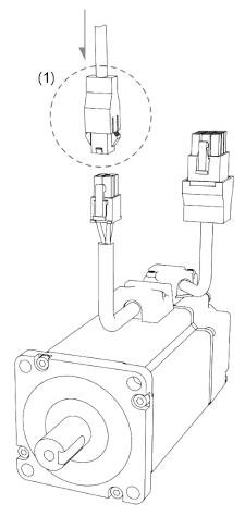
Note: pin assignments of the A3 and A2 model are the same. For easier wiring, A3's connector illustration (angle of viewing) is changed, which is different from that of A2.
