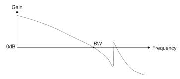
If you know the resonance frequency, the Notch filter can eliminate the resonance directly. The frequency range of the notch filter is 50-5000 Hz and the suppression strength is 0-32 dB. If the frequency does not meet the Notch filter conditions, then using the low-pass filter to reduce the resonance is suggested.
