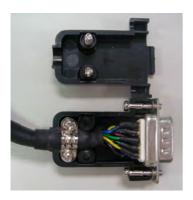
(2) Install the connector with shielding into the plastic case as shown in the figure.
