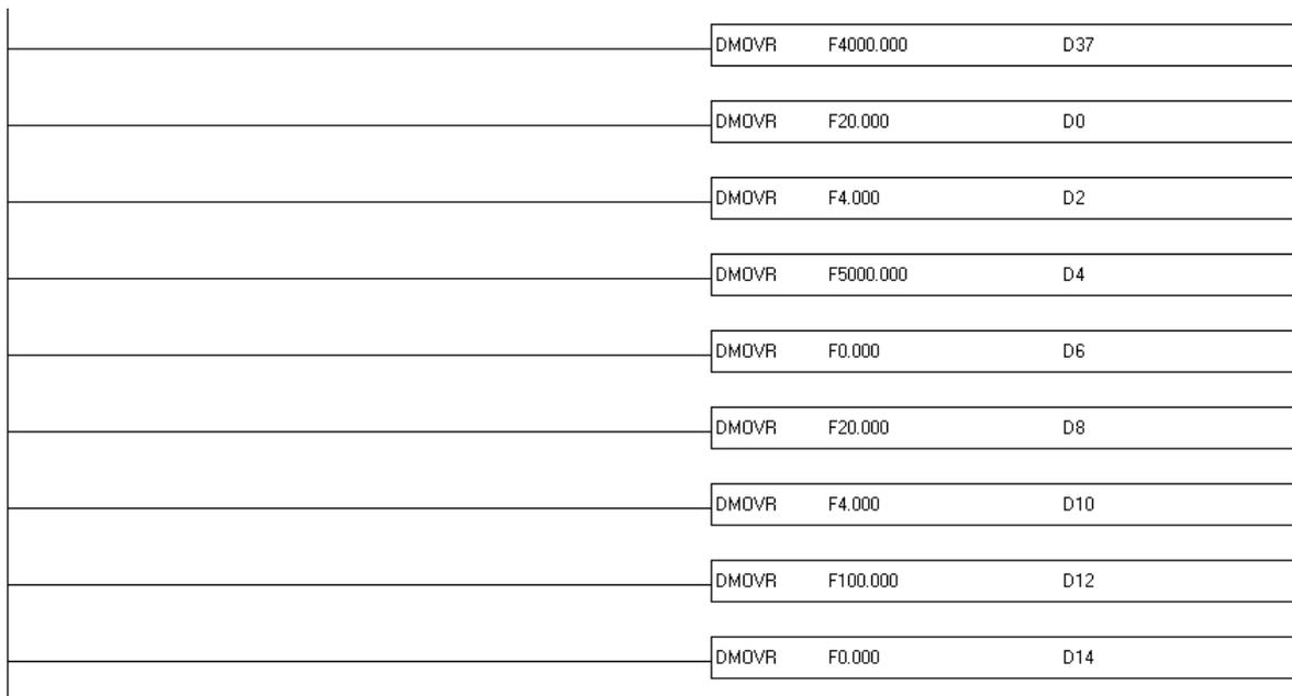
The value in D37 is digital full scale. In this example, the current input range for 04AD is 4 mA~20 mA, the digital conversion value range is 0~4000, and therefore the value in D37 is 4000.
