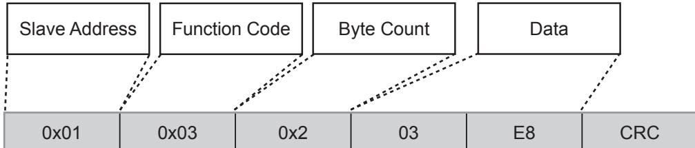
After receiving response from the power meter, Modbus Master acquires the value of currents from the primary-side current transformer (register address 0x000E), which is 1000.
