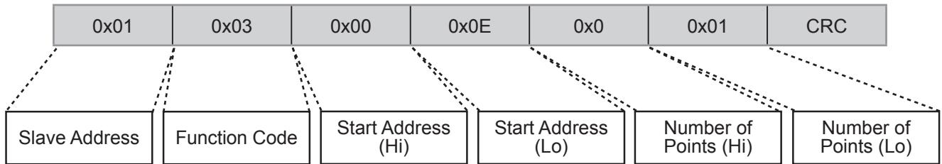
The packet format for Response responded by Modbus Slave (power meter) is as follows:
