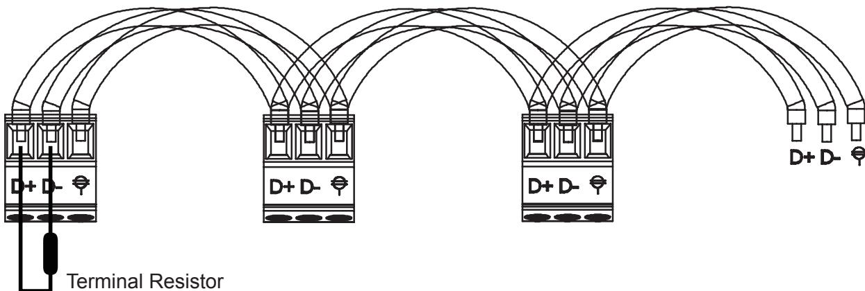
The D+ communication terminal for all devices should be connected on the same twisted pair cable.
