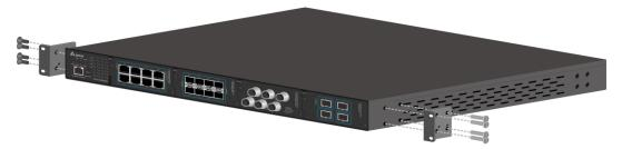
Step2: With front brackets orientated in front of the rack, nest front and rear brackets together.
