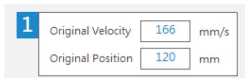
《 Fig. 3-2-1-1 》 Working origin condition setting
