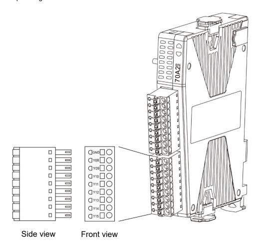
Mark Description **GND** Power ground of Port 1 Y08 1st set of output of Port 1 Y09 2<sup>nd</sup> set of output of Port 1 Y10 3<sup>rd</sup> set of output of Port 1 Y11 4th set of output of Port 1 Y12 5<sup>th</sup> set of output of Port 1 6th set of output of Port 1 Y13 7<sup>th</sup> set of output of Port 1 Y14 Y15 8th set of output of Port 1
