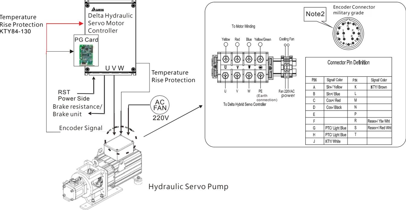
Note 2: The signal of KTY840-130 temperature rise protection is integrated into the encoder.
