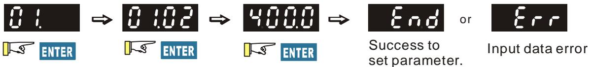
NOTE :In the parameter setting mode, you can press **ENTER** to return the selecting mode.
