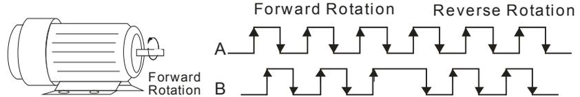
2: Phase B leads in a forward run command and phase A leads in a reverse run command.
