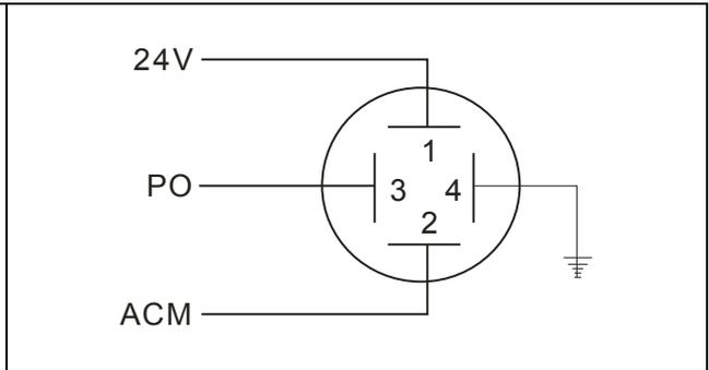
Current type pressure Sensor => Pin1: 24V , Pin2: PO , Pin3: N/A
