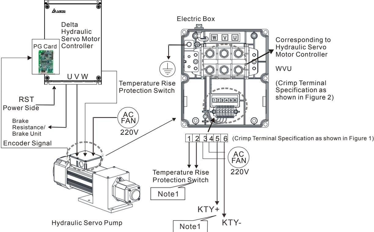
Note 1: After week 06 of year 2016, the temperature rise protection has been modified from On/Off switch (terminal 1 and 2) to KTY84-130 (terminal 5 and 6). Therefore the wiring method between the temperature rise protection and the hydraulic servo motor is different.
