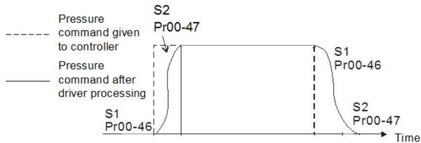
**00-48****Pressure Command Rising/ Descending S1 Curve**Control mode **VF FOC PG FOC PM**
