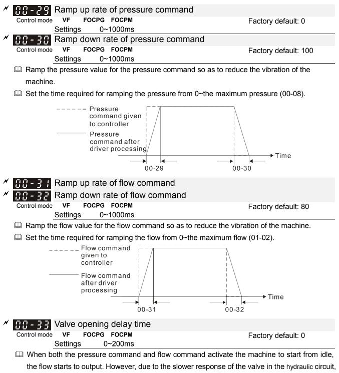
the sudden surge of the pressure may occur. The pressure may recover to normal till the valve is fully opened. To avoid the aforementioned effect, set this parameter to increase time for the flow output delay.
