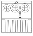
%2 Braking resistor 1500W 13 $\Omega$
