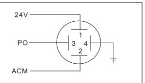
Current type pressure Sensor => Pin1: 24V , Pin2 : PO , Pin3 : N/A
