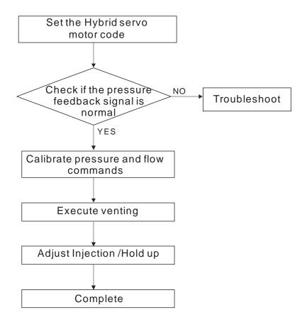
\*The firmware version is 2.04 and above, just proceeds the process to set up HES ID code. \*The firmware version is 2.05 and above, starts from "Execute venting". Chapter 3 Flow of machine Adjustment | HES Series
