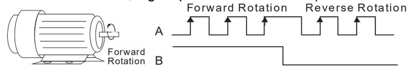
4: Phase A is a pulse input and phase B is a direction input. (low input=forward direction, high input=reverse direction).
