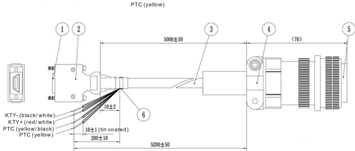
The colors mentioned in the Connector Pin Definition table are only the colors of lines inside the motor. They are not the colors of the lines on the encoder CBHE-E5M
