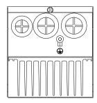
%2 Braking resistor 1500W 5.8 $\Omega$  Unit: min
