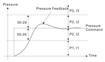
Adjust the Kp value to a proper level first, and then adjust the Ki value (time). If the pressure has overshoot, adjust the kd value.
