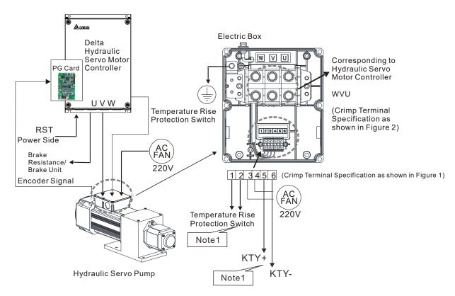
Note 1: After week 06 of year 2016, the temperature rise protection has been modified from On/Off switch (terminal 1 and 2) to KTY84-130 (terminal 5 and 6). Therefore, the wiring method between the temperature rise protection and the hydraulic servo motor is different.
