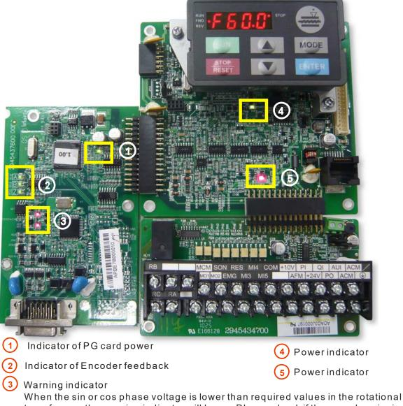
When the sin or cos phase voltage is lower than required values in the rotational transformer, the warning indicator will be on. Please check if the encoder wire is connected correctly. If it happens in operation, please check for any interference.
