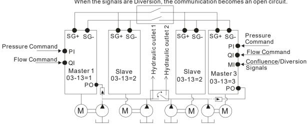
When the signals are Confluence, the communication will be a short circuit. When the signals are Diversion, the communication becomes an open circuit.
