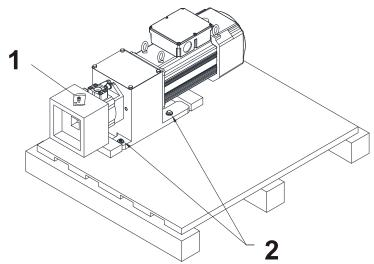
STEP 3: Lift the drive by using two lifting holes.
