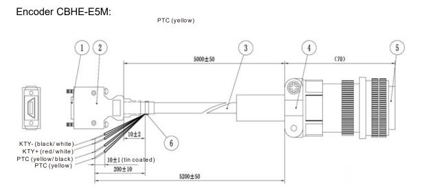
The colors mentioned in the Connector Pin Definition table are only the colors of lines inside the motor. They are not the colors of the lines on the encoder CBHE-E5M
