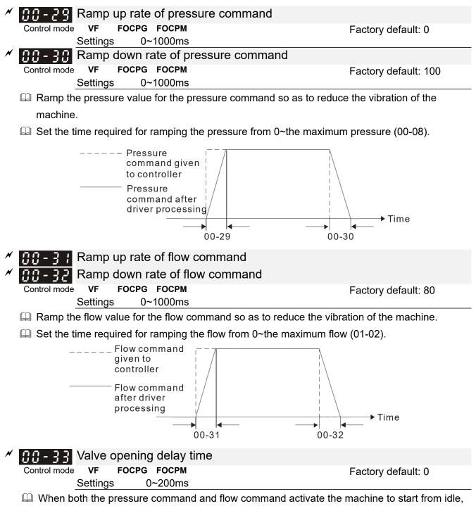
When both the pressure command and flow command activate the machine to start from idle, the flow starts to output. However, due to the slower response of the valve in the hydraulic circuit, the sudden surge of the pressure may occur. The pressure may recover to normal till the valve is fully opened. To avoid the aforementioned effect, set this parameter to increase time for the flow output delay.
