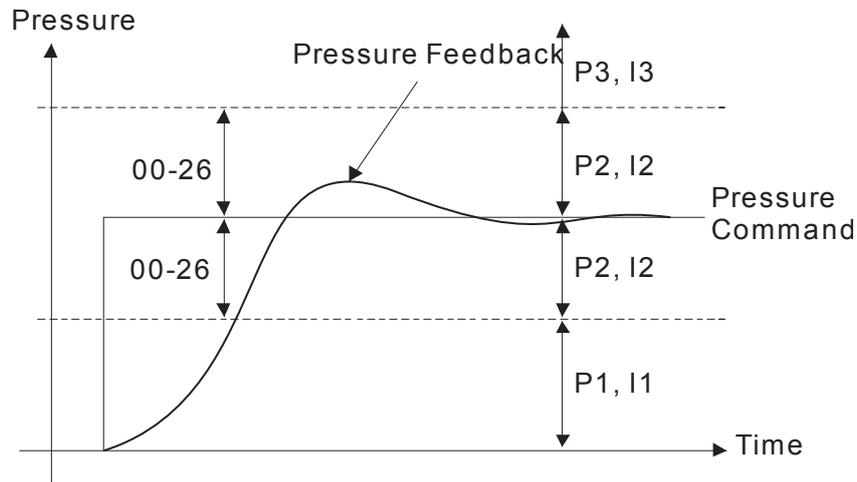
Adjust the  $K_p$  value to a proper level first, and then adjust the  $K_i$  value (time). If the pressure has overshoot, adjust the  $K_d$  value.
