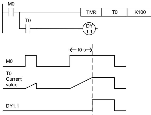
When M0 is on, the current value of the timer T0 increases by 100 ms, and once the current value equals the set value K100 (10 seconds), the output coil T0 is on. When M0 is off or the power is off, the current value of the timer T0 resets to 0 and the output coil T0 is turned off.
