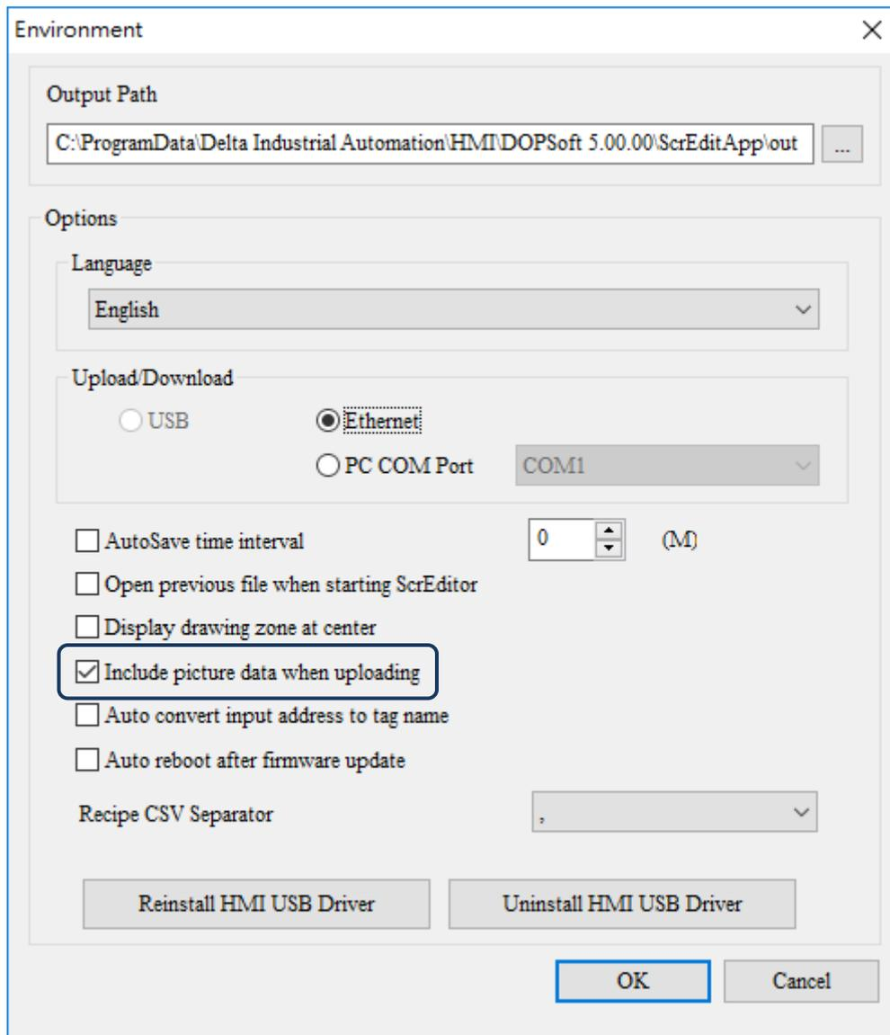
Figure 4.1.2.7 Include picture data when uploading
