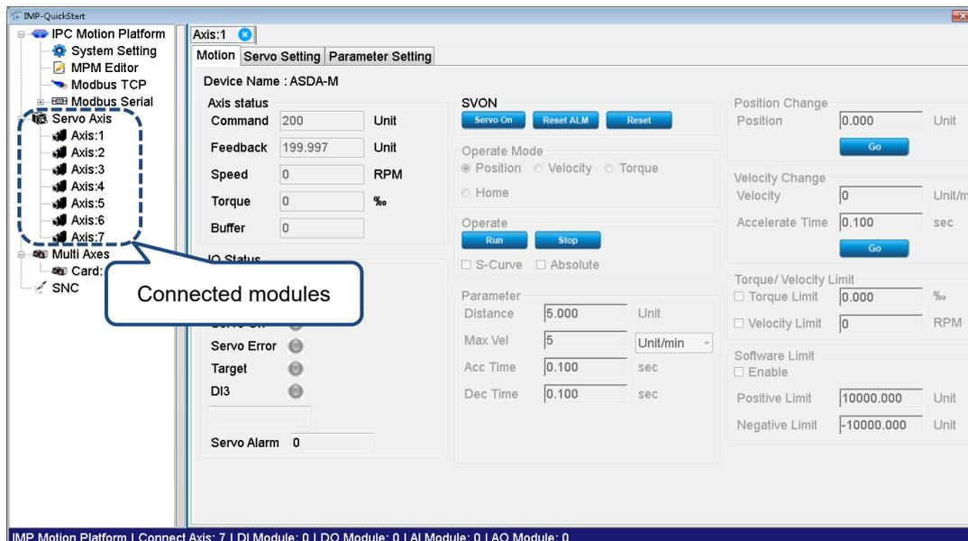
Figure 3.3.1.1 Single-axis control screen
