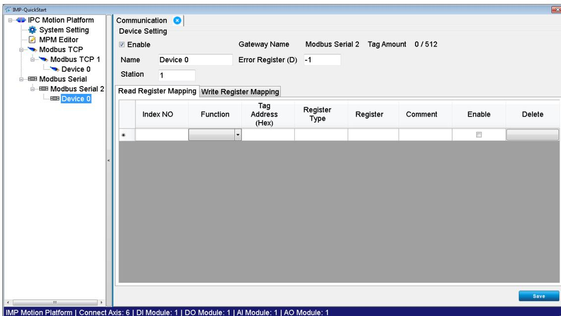
Figure 8.1.1.2 Modbus / Serial connection device setting
