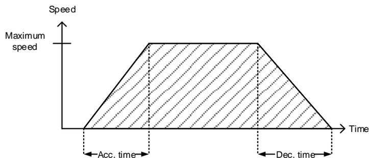
Figure 5.2.2.2 Acceleration / deceleration time setting
