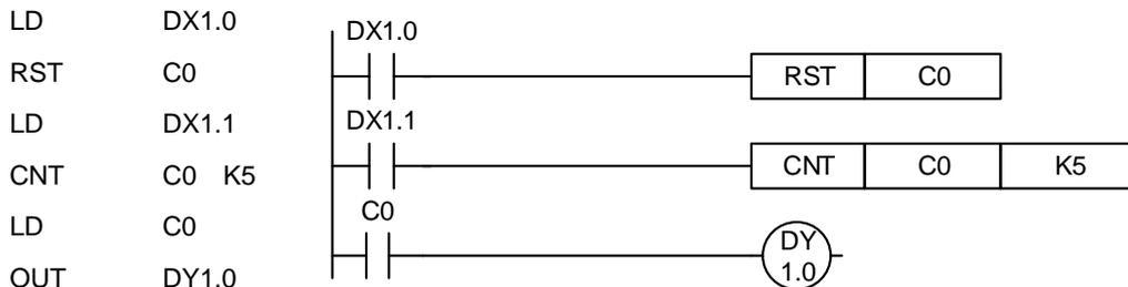
When DX1.0 is on, execute the RST command, then the C0 count resets to zero and the counter C0 bit is off. When DX1.1 switches from off to on, the current value of counter C0 increments by 1. When the count of counter C0 reaches the set value K5, the counter C0 output bit is on and the current value of C0 equals the set value K5. After that, C0 no longer receives the triggering signal of DX1.1 and the current value of C0 remains at K5. See the diagram below for the example:
