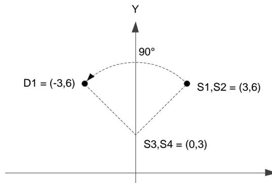
Example: rotate the coordinate (3, 6) by 90 degrees based on (0, 3) as the center and store the result (-3, 6) in the four registers starting with D1.
