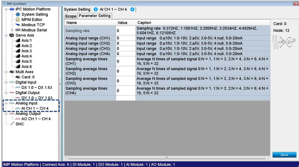
Figure 3.2.6.1 Parameter setting screen for the analog input module
