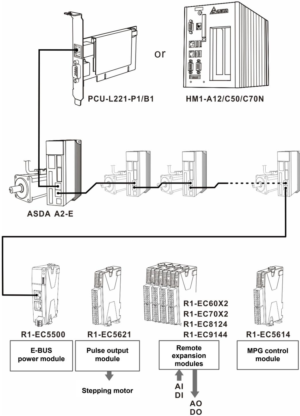
Figure 1.2.2 EtherCAT communication architecture diagram
