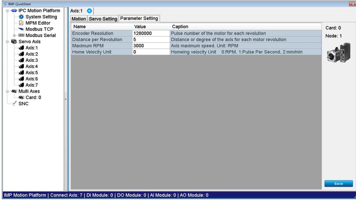
Figure 3.2.2.3 Pulse module parameter setting screen
