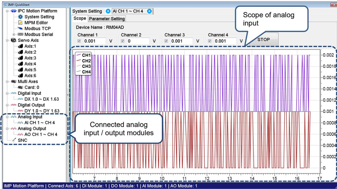
Figure 3.2.5.1 Analog input CH 1 - CH 4 view screen
