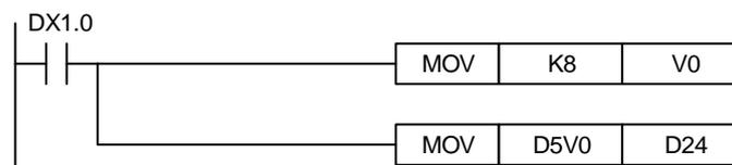
When DX1.0 is on, V0 = 8, D5V0 = D(5+8) = D13, the content of D13 is moved to D24.
