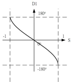
Example: perform  $\text{COS}^{-1}$  operation on the value of 0.5 and store the result in register D12. After the execution, the values of registers D13 and D12 are 60.0 (floating point format).
