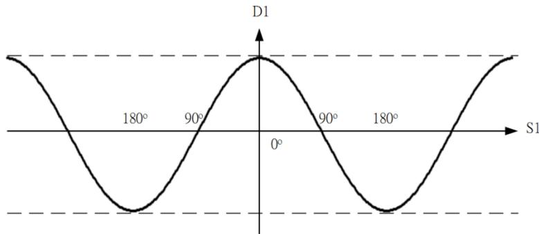
Example: set the values of registers D11 and D10 to 45.000 (floating point format), perform COS operation on the contents of register D10, and store the result in register D12.
