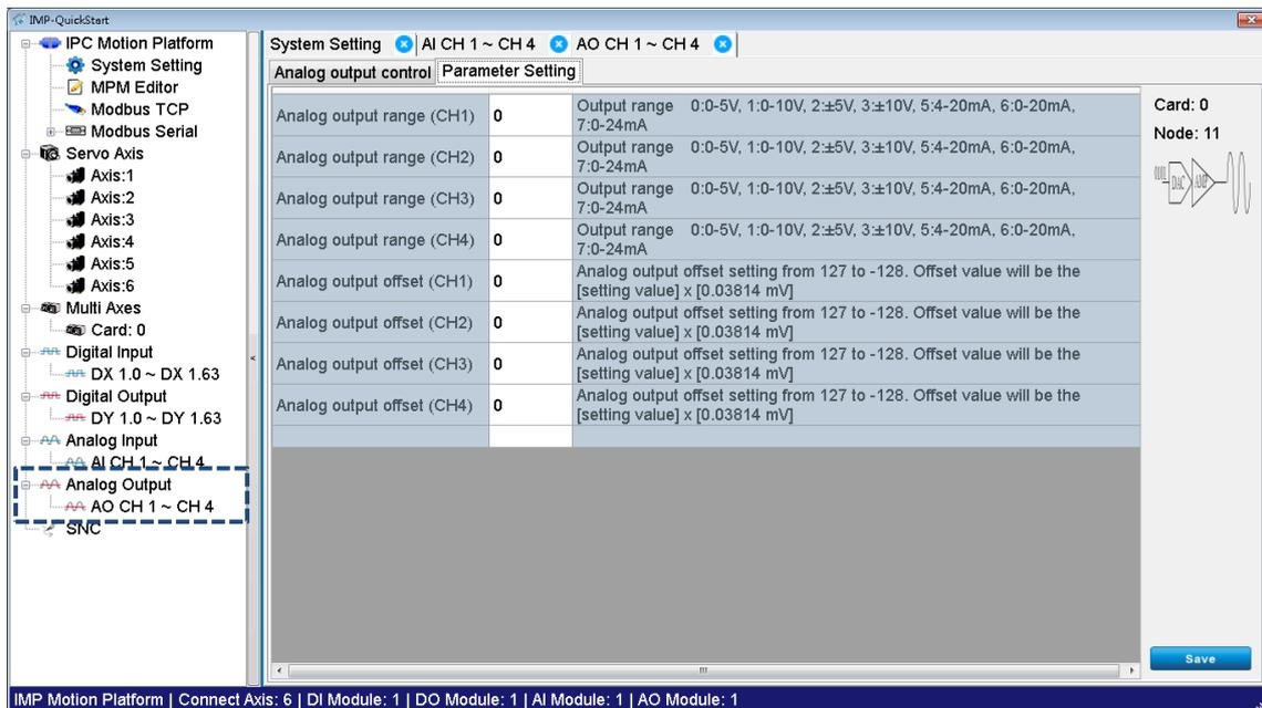
Figure 3.2.6.2 Parameter setting screen for the analog output module
