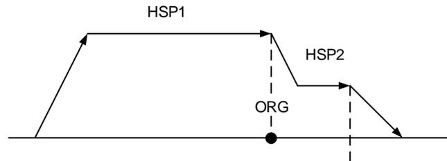
Figure 5.2.2.1 Homing speed switching
