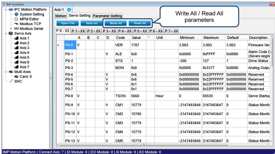
Figure 3.3.2.2 Read the servo drive parameters
