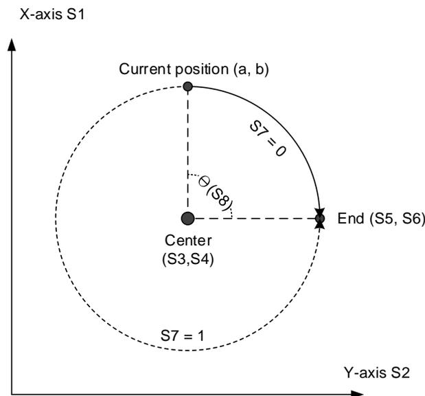
Example: Axis X and Axis Y move to the position (-15, 15), make a 1/4 arc motion around the center at (0, 0) in clockwise direction, and stop at the position (15,15). Then, this MPM ends.
