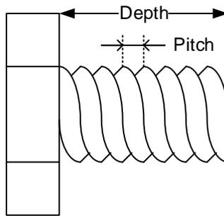
Example: the tapping speed of rotation axis X is 100 rpm, and at each turning cycle of axis X, the corresponding axis Y feeds 7 mm (pitch). The total feeding distance of axis Y is 70 mm. When the tapping finishes, axis X and axis Y decelerate to stop and delay for 65 ms, then the rotation axis X carries out the retraction at 160 rpm in reverse direction.
