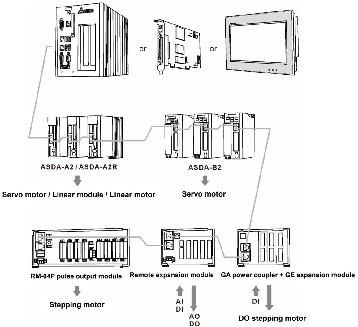
Figure 1.2.1 DMCNET architecture diagram
