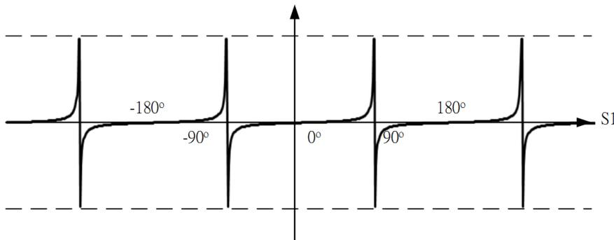
Example: set the values of registers D11 and D10 to 45.000 (floating point format), perform TAN operation on the contents of register D10, and store the result in register D12. After the execution, the values of registers D13 and D12 are 1.0 (floating point format).
