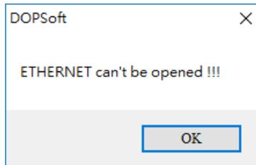
The following error message pops up if the connection cable is removed or the communication is interrupted during the download process.
