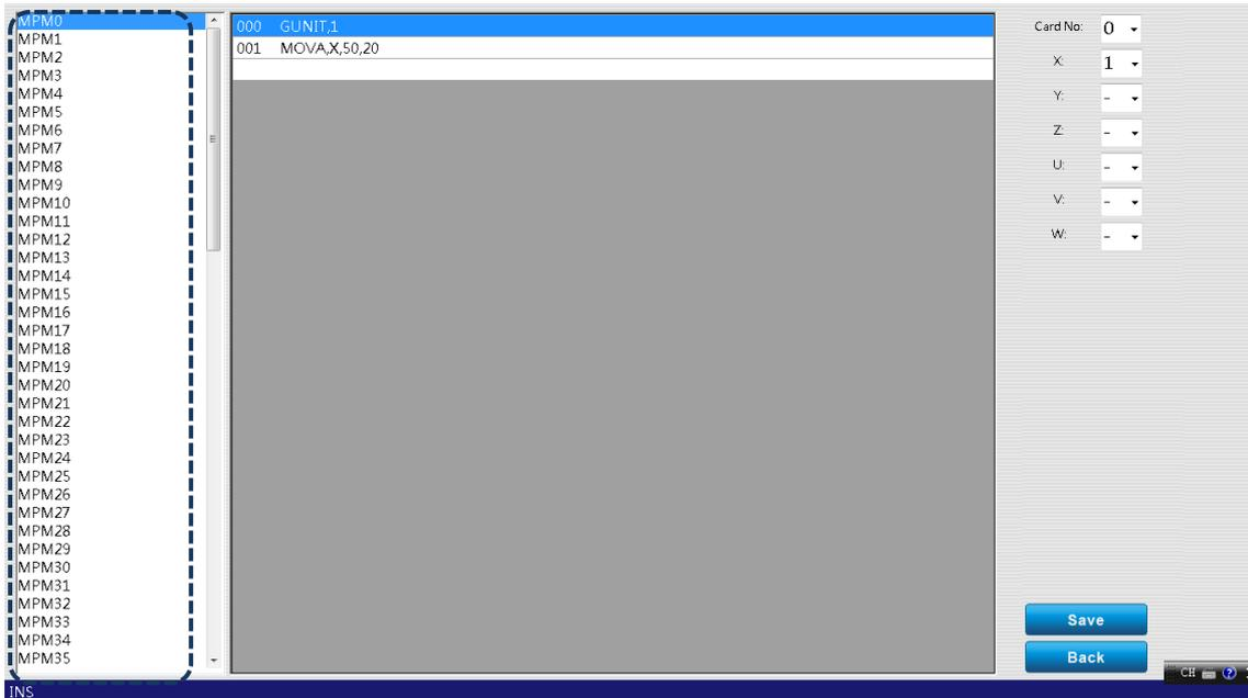
2. Select the card number and axis. The range of the card number is between 0 and F; the available axes are X, Y, Z, U, V and W, which you can set the corresponding node number.
