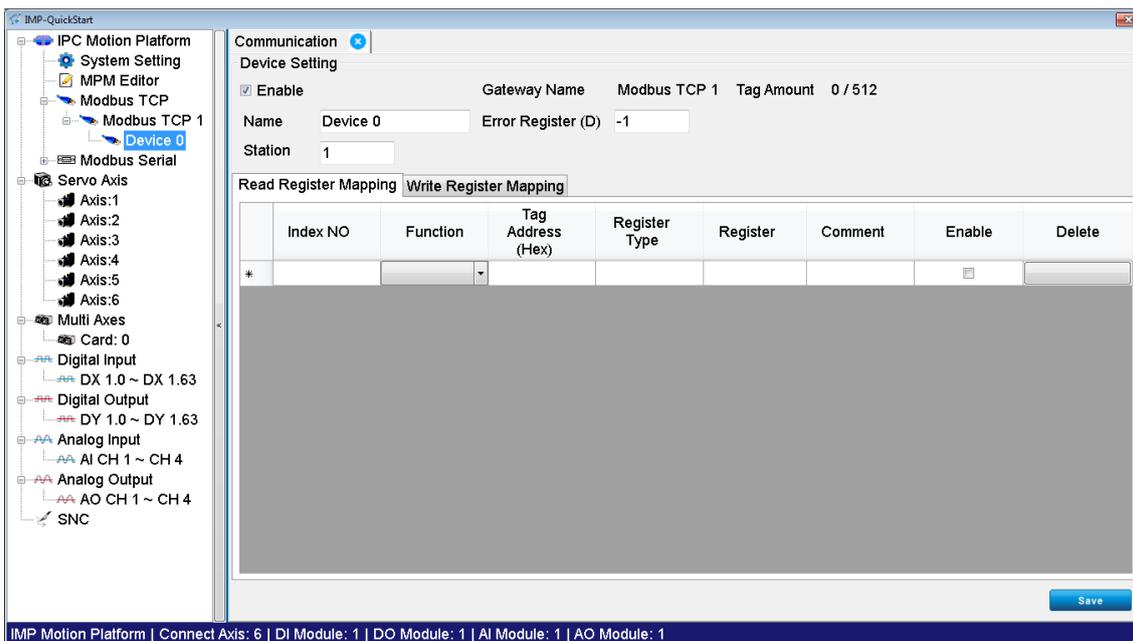
Figure 8.1.1.2 Modbus / TCP connection device setting
