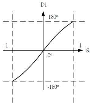
Example: perform  $TAN^{-1}$  operation on the value of 0.5 and store the result in register D12. After the execution, the values of registers D13 and D12 are 26.57 (floating point format).
