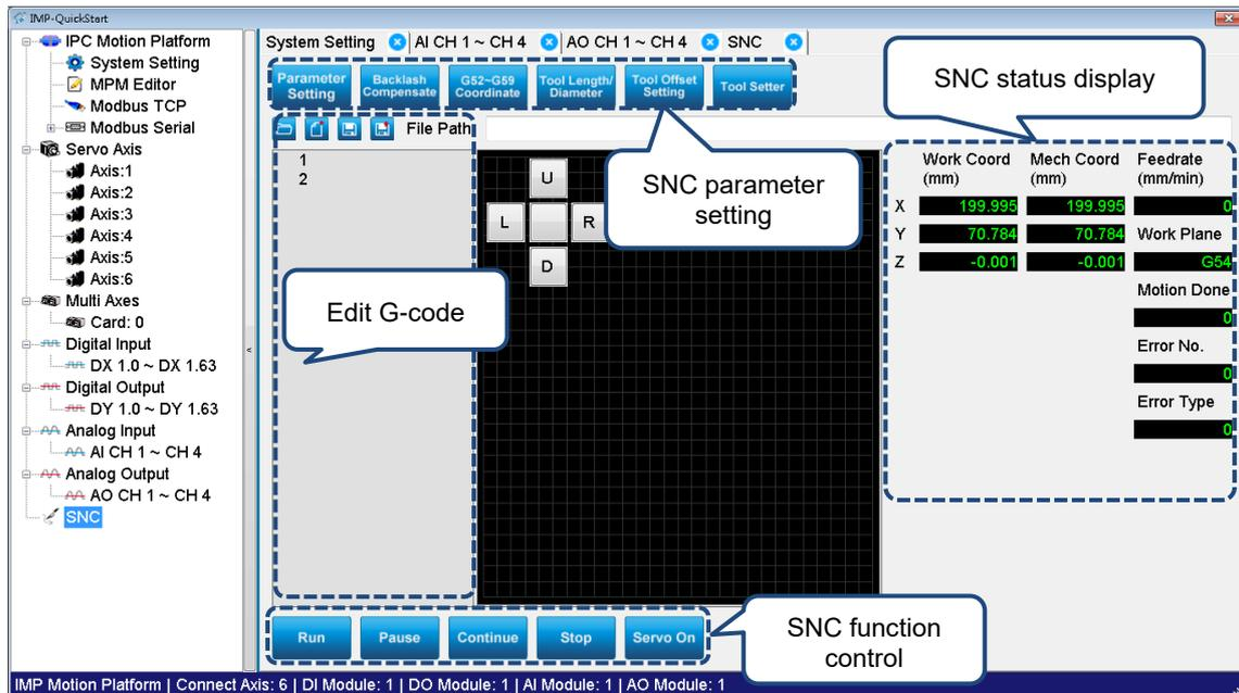
Figure 3.2.7.1 Interface of software numerical control
