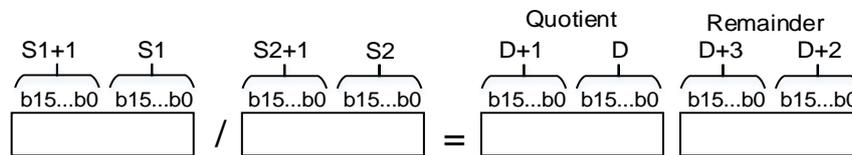
Example: 16-bit D0 is divided by 16-bit D10 and the result is the quotient of 32-bit. The upper 16-bit is saved in D21, the lower 16-bit is saved in D20, and on / off of the leftmost bit indicates the positive and negative result.
