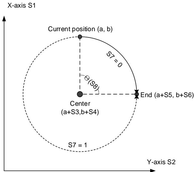
Example: Axis X and Axis Y move to the position (-15, 15), make a 1/4 arc motion around the center at (0, 0) in clockwise direction, and stop at the position (15, 15). Then, this MPM ends.
