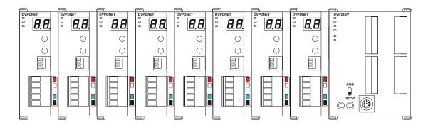
The index of DVPDNET-SL is its unit number. The first DVPDNET-SL on the left hand side of DVP-SV is No. 1, the following DVPDNET-SL modules are No. 2, No. 3, No. 4 and so on.
