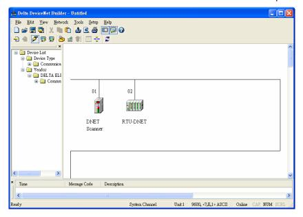
5> Double click on RTU-DNET (node 02), and the "Node Configuration..." dialog box will appear.
