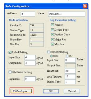
6> Click on "IO Configure..." button in "Node Configuration" dialog box, and you will then see "RTU Configuration" page where you click on "Scan IO" button and "Warning" dialog box will appear. Click "OK" then DeviceNet Builder will detect the devices connected to RTU-DNET as below.
