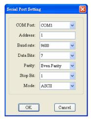
2> Set up the communication parameters in the PC and DVP-SV, e.g. the communication port, address, baud rate and communication format. Click on "OK" after configuration is finished.
