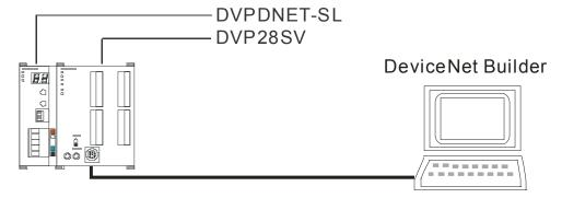
2) Open DeviceNet Builder software and select "Setup" => "Communication Setting" => "System Channel". And then the following dialog box appears.
