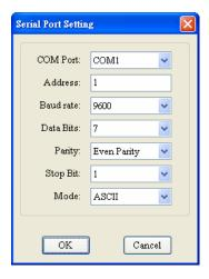
3) Set up the communication parameters in the PC and DVP-SV, e.g. the communication port, address, baud rate and communication format. Click on "OK" after configuration is finished.
