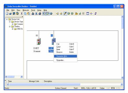
6) Set parameter 5 as "Enable" and select the baud rate in parameter 6 in the following page. Click on "Download" to download the newly set parameter value to DVPDNET-SL (Slave).
