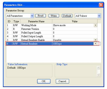
7) After download is completed, set DVPDNET-SL (Slave) 's function switch: DR0 and DR1 as ON. And then repower PLC to finish the setting of the extended baud rate.
