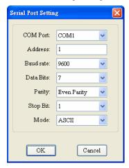
3) Set up the communication parameters in the PC and DVP-SV, e.g. the communication port, address, baud rate and communication format. Click on "OK" after configuration is finished.
