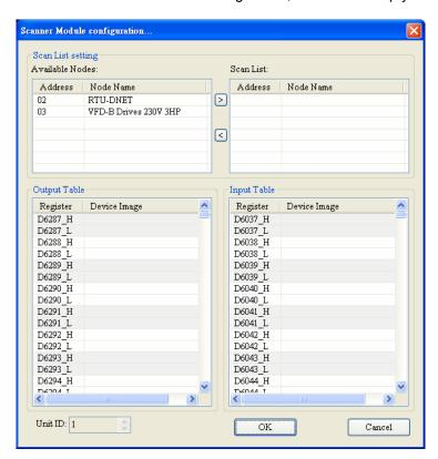
2> (2) Move the slave devices on DeviceNet in the "Available Nodes" list on the left side to the "Scan List" on the right side. Select a node and click on. Follow the steps to move all the nodes to the scan list.
