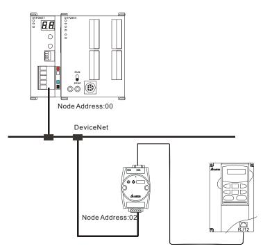
Note: IFD9502, a Delta DeviceNet slave module can connect VFD AC motor drive to DeviceNet network.
