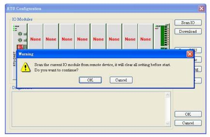
7> Because no special module is connected to the right side of RTU-DNET, "None" will show in the location of the special module in the following window. The point number for X and Y are both 0.Then click on "Gateway setting".
