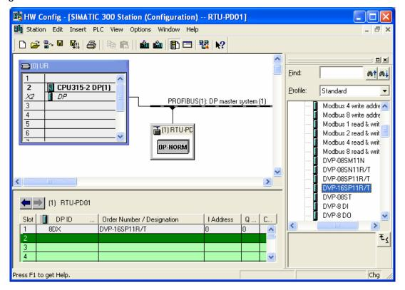
6. Configure other slots as configuring Slot 0. To configure, select one of the slots and double click on the items to be configured in the right-hand side column. Apply it to configure Slot 0 ~ Slot 4.
