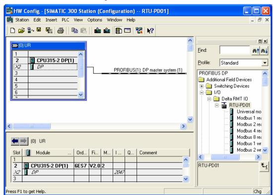
3. We can then see RTU-PD01 in the right-hand side column. RTU-PD01 is the module added.
