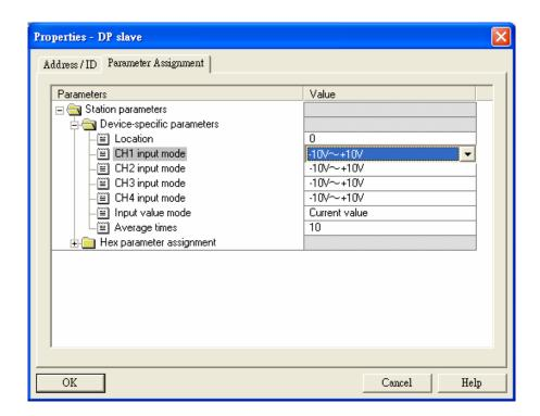
9. Double click the configured Slot 3 in "HW Config" window to open the dialog box in the figure below. Refer to 8.3.3 for the definition of every parameter in this dialog box.
