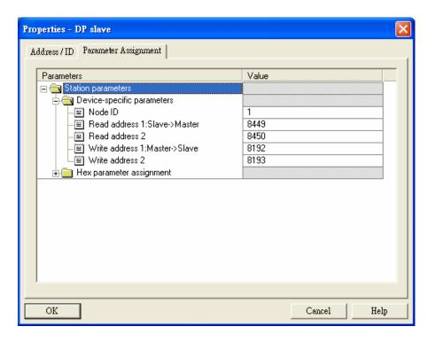
11. After all the configuration items for RTU-PD01 are set, double click the RTU-PD01 slave on the PROFIBUS DP bus in "HW Config" window to open the dialog box in the figure below. Refer to 8.1 for the definition of every parameter in this dialog box.
