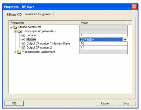
10. Double click the configured Slot 4 in "HW Config" window to open the dialog box in the figure below. Refer to 8.3.4 for the definition of every parameter in this dialog box.
