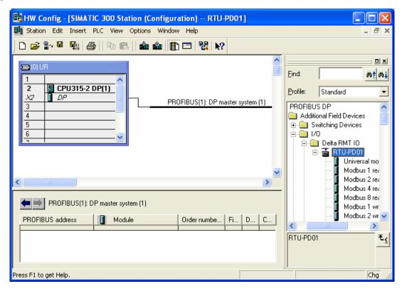
2. In the dialog box, select the address of RTU-PD01 slave. The address has to be the same as the setting of address setup switch on RTU-PD01. Click "OK".
