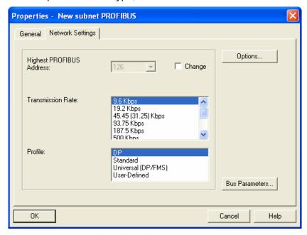
6. Confirm the communication speed and master address for PROFIBUS DP bus, then click "OK".
