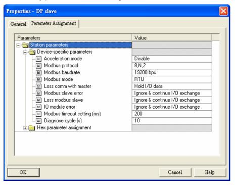
12. After all the parameters are set, download the parameters, and once the master is connected to RTU-PD01, the NET indicator on RTU-PD01 will constantly be On in green color.
