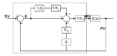
Figure 2 Control diagram for control mode 3/4 (S<sub>3</sub>+4 is K3/K4.)
