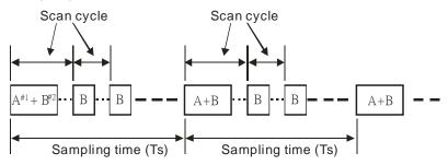
Note: #1> Time it takes for the algorithm to be calculated during the execution of PID (approximately 72 us)  $#2 \rightarrow$  Time it takes for PID to be executed without the performance of the algorithm (approximately 8 us)
