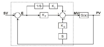
Figure 1 Control diagram for control mode 0/1/2/5 (S<sub>3</sub>+4 is K0/K1/K2/K5.)
