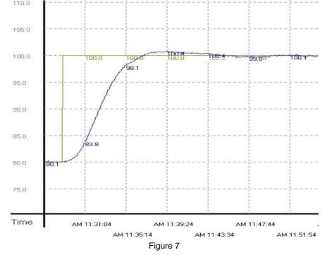
In Figure 7, the users can see that the purpose of controlling the temperature can still be met after the parameters adjusted for 80°C are applied to 100°C, and it does not take much time to control the temperature.
