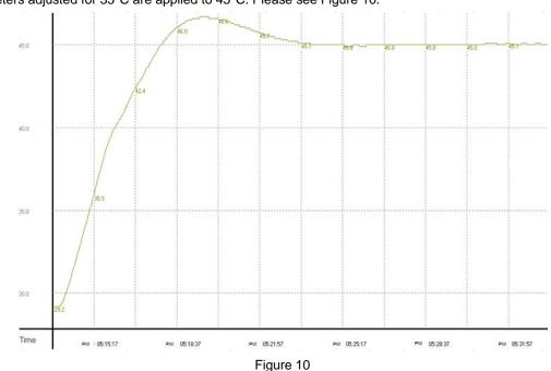
The parameters adjusted for 35°C are applied to 45°C. Please see Figure 10.
