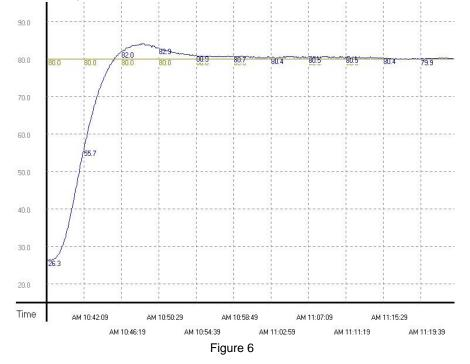
The experimental result of using the parameters after the adjustment for temperature control is shown in Figure 6.
