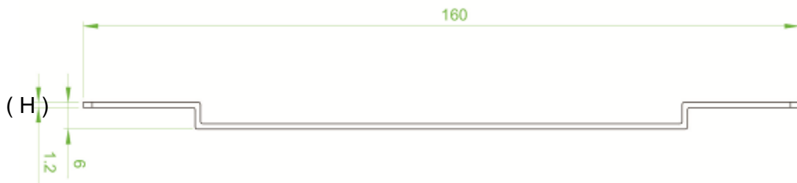
▲ Side view of base retainer
