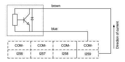
Wiring example: The proximity switch of PNP two-wire system PNP 2 wire system proximity switch
