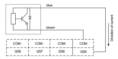
Wring example: The proximity switch of NPN three-wire system
