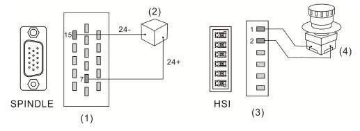
(1) & (3) EMG connector (Female); (2) Power supply; (4) Emergency stop button
