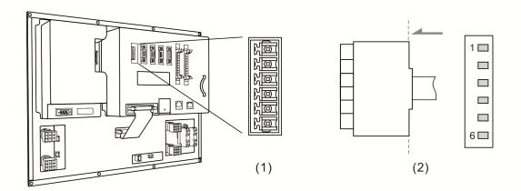
(1) Remote I/O connector on NC controller (Female); (2) Remote I/O connector on the module (Male)
