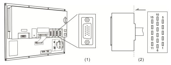
(1) Spindle connector on NC controller (Female); (2) Spindle connector (Male)
