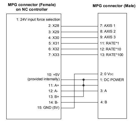
Wiring for differential type MPG (EHDW-BE6SI):
