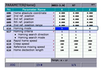
2. Once the parameter is set, execute homing procedure of absolute motors by going to screen of [DGN] > [System monitoring] > [Servo monitoring]. See the figure below.
