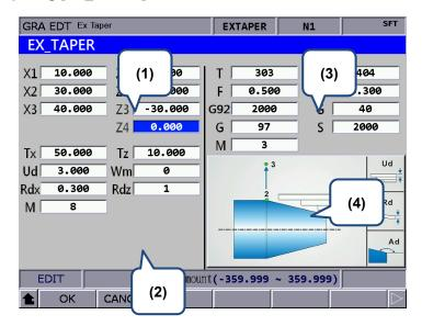
(1) Input the coordinates of each step point (Fields with blue texts can be left blank and it means the point does not exist.)
