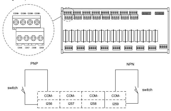
Wiring example: The proximity switch of NPN two-wire system NPN 2 wire system proximity switch
