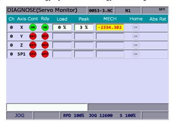
3. To exeute homing procedure, the system setting has to be done in **JOG** or **MPG** mode. Firstly, change the mechanical coordinate to the proper position. Then, enter 1 and press **ENTER**, the homing is complete. Meanwhile, the origin indicator will light up and mechanical coordinates displays 0; it means this axis has completed the homing procedure.
