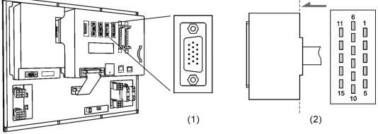
(1) AXIS1 ~ 4 connector on NC controller (Female); (2) AXIS1 ~ 4 connector (Male)
