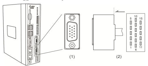
(1) RS-485 connector on NC controller (Female); (2) RS-485 connector (Male)
