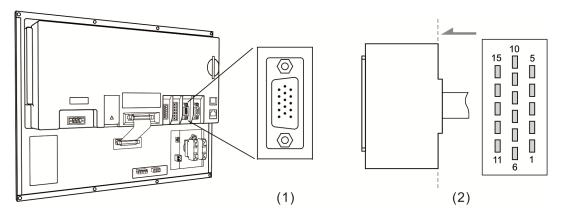
(1) RS-485 connector on NC controller (Female); (2) RS-485 connector (Male)
