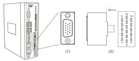
(1) Spindle connector on NC controller (Female); (2) Spindle connector (Male)
