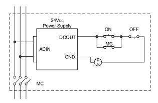
If the Power ON button is pressed, the circuit is closed between PIN ONA1 and ONA2; if the Power OFF button is pressed, the circuit is open between PIN OFFB1 and OFFB2.
