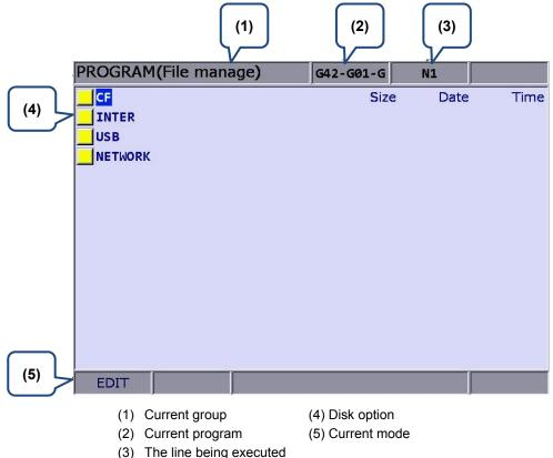
Set the system to **Edit mode**. Then, press the **PRG** key in the primary control panel to enter the screen of [Program].
