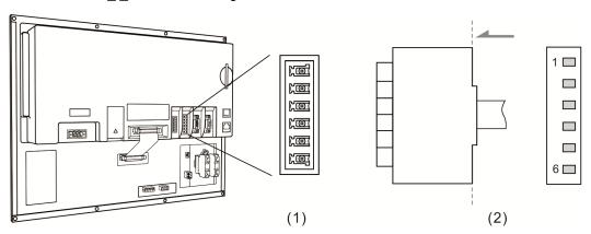
(1) HSI connector on NC controller (Female); (2) HSI connector (Male)
