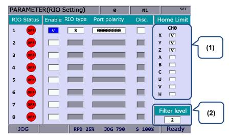
(1) Axis selection. The positive, negative and origin DI of Axis X ~ A are input by port AXIS1~4 of the controller. According to the axis number and name selected, starting from X256, each axis occupies three DI points, positive, negative and origin respectively.
