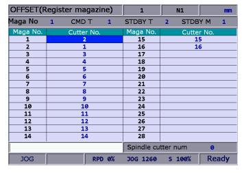
Set position 1 = 2, and tools ID 1 and 2 in tool magazine 1 and 2 exchanges with each other.
