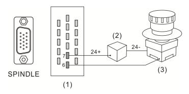
(1) EMG connector (Female); (2) Power supply; (3) Emergency stop button
