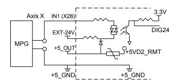
The wiring varies with the signal types of the MPG (only support 100 PPR type), which includes single-ended (EHDW-BA6SI) and differential (EHDWBE6SI).
