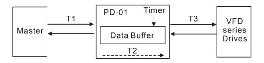
T1 depends on the actual transmission speed and the type of master in use.
