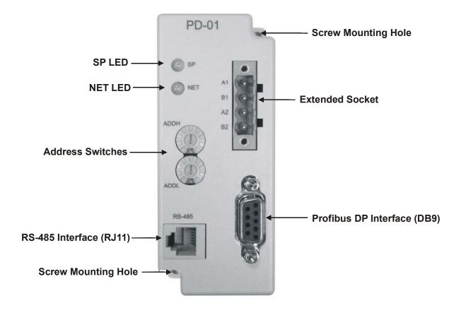
SP LED: Indicating the connection status between Drives and PD-01 NET LED: Indicating the connection status between PD-01 and PROFIBUS-DP Address Switches: Setting the address of PD-01 on PROFIBUS-DP network RS-485 Interface (RJ11): Connecting to VFD Drives, and supply power to PD-01 PROFIBUS-DP Interface (DB9): 9-PIN connector that connects PD-01 to PROFIBUS-DP network
