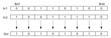
The steps for XOR operation when more than 2 input parameters exist are: The XOR result of In1 and In2 is got first; then the XOR operation of the previous result and In3 is conducted and so on. Finally, the XOR operation of the previous XOR result and InN is processed. The XOR result of In1 and In2 is Out\_Temp and the XOR result of Out\_Temp and In3 is Out as shown below.
