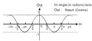
Users can choose different data types for the input parameter in this instruction. But the data type of the output parameter is restricted to LREAL. An error will occur during the compiling of the software if the data type of the output parameter is not LREAL.
