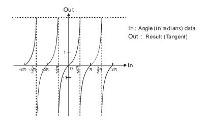
Users can choose different data types for the input parameter in this instruction. But the data type of the output parameter is restricted to LREAL. An error will occur during the compiling of the software if the data type of the output parameter is not LREAL.
