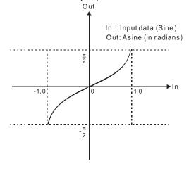
Users can choose different data types for the input parameter in this instruction. But the data type of the output parameter is restricted to LREAL. An error will occur during the compiling of the software if the data type of the output parameter is not LREAL.
