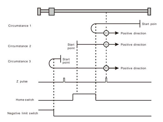
Homing depending on the home switch, negative limit switch and Z pulse (1): mode 11)
