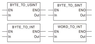
The rule for the conversion of bit-string data into integer data is consistent with that for the conversion of bit-string data into bit-string data.
