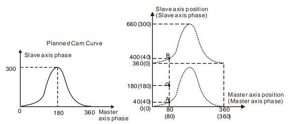
There are three modes of *StartMode* for selection: the shortest way (mcRampInShortest), positive direction (mcRampInPositive) and negative direction (mcRampInNegative). Users can select the right engagement mode according to actual need.
