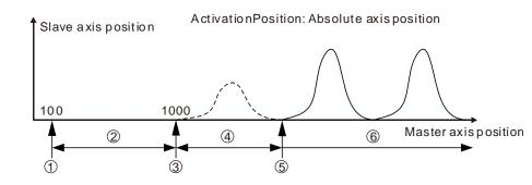
**Stage 1:** Trigger and execute the MC\_CamIn instruction. The master axis absolute position is 100 at the moment.
