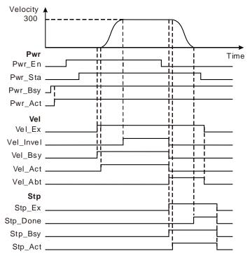
When Vel \_Ex changes to TRUE, Vel \_Bsy changes to TRUE; one cycle later, Vel \_Act changes to TRUE and the servo motor starts moving in the positive direction. When the speed of the servo motor reaches the target velocity, Vel \_Invel changes to TRUE.
