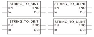
For the string-to-integer conversion, the string is required to be the integer value such as '123', '-123' and '+123'. The string like 'M123' is not allowed to convert to the integer. The conversion examples are shown in the following table.
