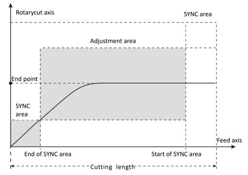
After the instruction "APF\_RotaryCut\_Out" is started up, the system will use the curve to make the rotary cut axis break away from the rotary cut state. Eventually, the knife stops at the end position as shown in the figure above.
