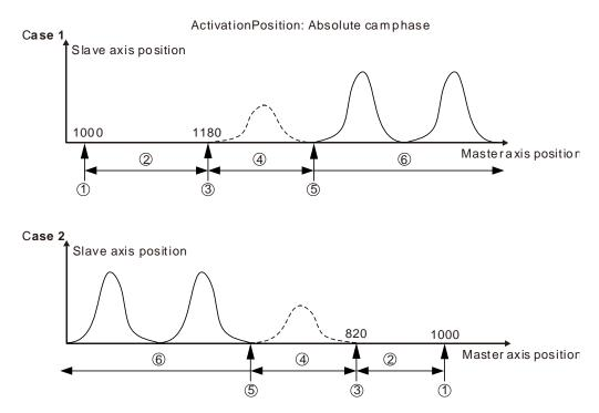
**Stage 1:** Trigger and execute the MC\_CamIn instruction. The master axis absolute position is 1000 at the moment. (The absolute cam phase is 280)
