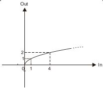
Users can choose different data types for the input parameter in this instruction. But the data type of the output parameter is restricted to LREAL. An error will occur during the compiling of the software if the data type of the output parameter is not LREAL.
