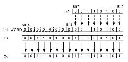
If the data type of an input variable is BOOL, the data types of all input and output variables are required to be BOOL. Otherwise, an error will occur in the compiling of the software.
