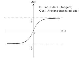
Users can choose different data types for the input parameter in this instruction. But the data type of the output parameter is restricted to LREAL. An error will occur during the compiling of the software if the data type of the output parameter is not LREAL.
