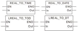
For the real number-to-time or date conversion, the real number is converted to the integer first and then the integer is converted to the time or date. For relevant contents, refer to the real number-to- integer conversion and integer-to-time or date conversion.
