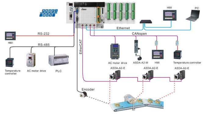
The figure above illustrates the peripheral devices which are connected to various ports of DVP-50MC series motion controller in the entire system. Refer to "Wiring, Communication Setting and Network Construction" for details on the functions of communication ports.
