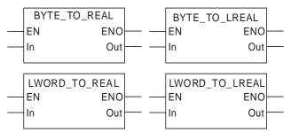
> The Bit-string data are converted into the Real-number data as the following table shows.
