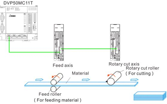
Note: The feed axis is to control the feed roller; the rotary cut axis is to control rotary cut roller with the knife mounted on the rotary cut roller. The rotary cut function is usually used for cutting of the thin material or the material of medium thinness and can be applied in packaging machine, cutting machine, punching machine, printing machine etc.
