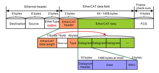
The EtherCAT port of the controller exchanges data with EtherCAT slaves according to COE (CANopen over EtherCAT) protocol. There are two kinds of transmission methods for the controller and slaves. One is cyclic data exchange based on the specified time cycle, called PDO (Process Data Object). The other is request-response data exchange, called SDO (Service Data Object).
