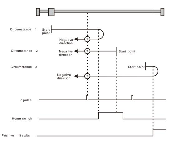
Homing depending on the home switch, positive limit switch and Z pulse (2: mode 7)
