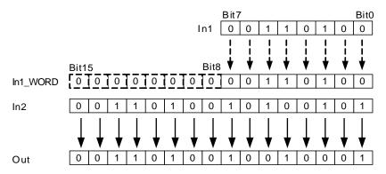
If the data type of an input variable is BOOL, the data types of all input and output variables are required to be BOOL. Otherwise, an error will occur in the compiling of the software.
