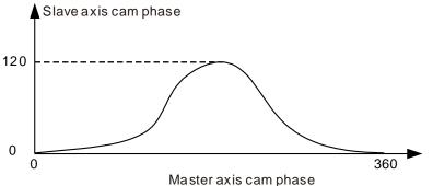
When the master axis and slave axis are both in absolute mode and the engagement begins, the master axis position and slave axis position are both 0. When there is no position offset and scaling (the offset and scaling are default values), the actual master axis position correspond to the actual slave axis position in the execution of the cam motion as shown in the following figure.
