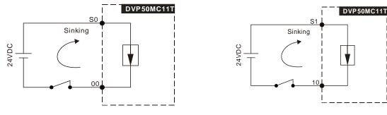
See relevant wiring circuits in the following figures.
