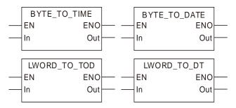
The rule for the conversion of Bit-string data into Time or Date data is the same as that for the conversion of the Bit-string data into unsigned integer data.
