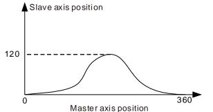
When the offset and scaling are not default values, the corresponding relationship between the actual master axis position and actual slave axis position are affected in the execution of the cam motion as below.
