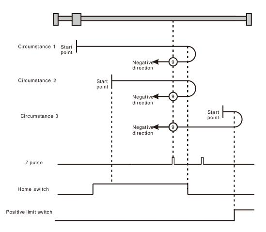
Homing depending on the home switch, positive limit switch and Z pulse (9: mode 9)
