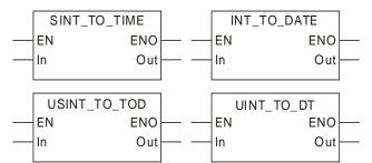
The rule for the conversion of the Integer data into the Time or Date data is the same as that for the conversion of the Integer data into the unsigned integer data.
