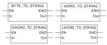
> The Bit-string data are converted into the String data as the following table shows.
