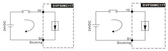
See the wiring circuit below:
