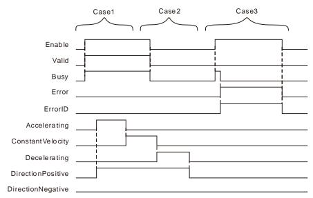
**Case 1:** When *Enable* changes from FALSE to TRUE, *Valid* and *Busy* change to TRUE and ConstantVelocity, Accelerating, Decelerating, DirectionPositive and DirectionNegative change to TRUE or FALSE according to the axis state.
