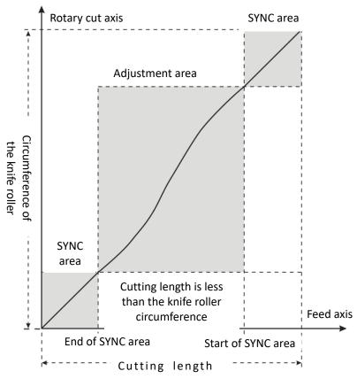
For the cutting of short material, rotary cut axis must accelerate first in the adjustment area, and then decelerate to the synchronous speed.
