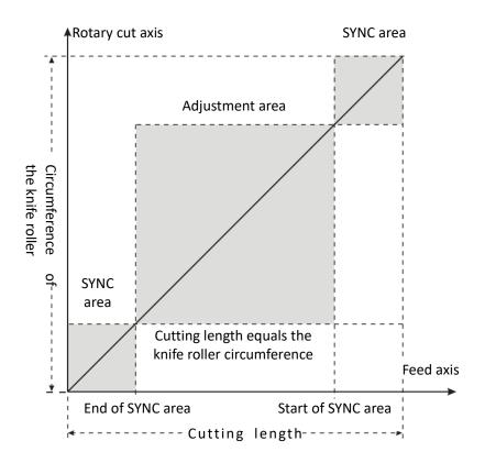
In this situation, the feed axis and rotary cut axis in SYNC area and non-SYNC area keep synchronous in speed. The rotary cut axis does not need to make any adjustment.
