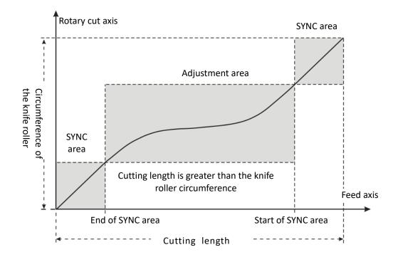
In this situation, the rotary cut axis should decelerate first in the adjustment area and then accelerate to the synchronous speed. If the cutting length is far greater than rotary cut roller circumference, the roller may decelerate to 0 and stay still for a while; and then accelerate up to the synchronous speed. The greater the cutting length is, the longer the roller stays.
