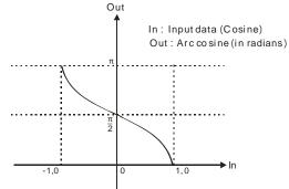
Users can choose different data types for the input parameter in this instruction. But the data type of the output parameter is restricted to LREAL. An error will occur during the compiling of the software if the data type of the output parameter is not LREAL.
