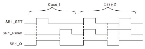
**Case 1:** When SR1\_SET is TRUE, SR1\_Q is TRUE. When SR1\_Reset is TRUE, SR1\_Q is FALSE. **Case 2:** SR1\_SET is given the priority when SR1\_SET and SR1\_Reset are both TRUE.
