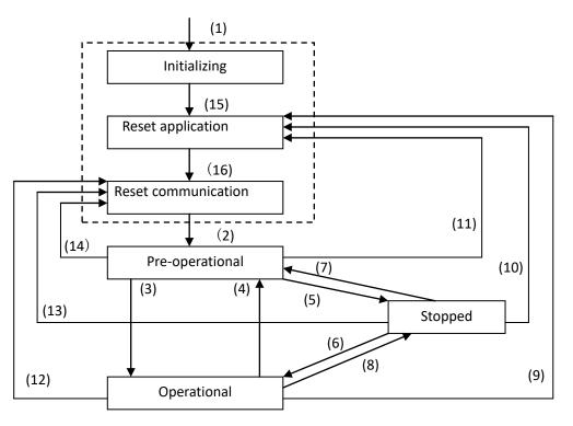
(1) After the power is supplied, the device automatically enters the initialization state.
