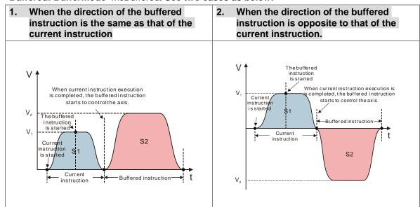
■ Buffered: Buffermode=mcBuffered. See two cases as below.
