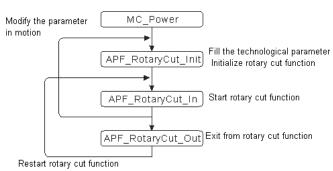
2. When the rotary cut function is performed, the rotary cut axis can only execute APF\_RotaryCut\_Out and MC\_Stop instruction and other instructions are invalid.
