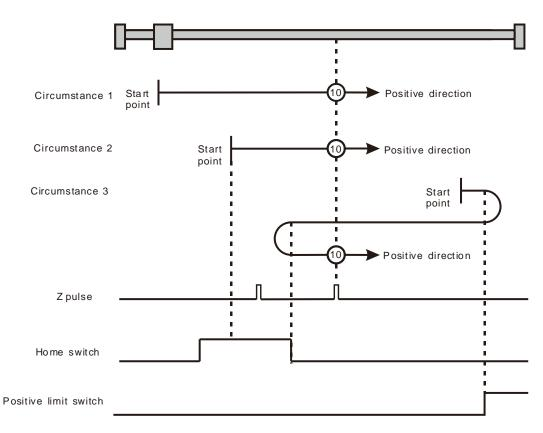
Homing depending on the home switch, positive limit switch and Z pulse (10): mode 10)
