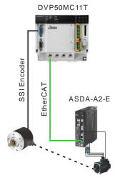
Specification for SSI Absolute Encoder Interface Wiring SSI encoder interface of DVP-50MC series motion controller and the wiring method are shown below.
