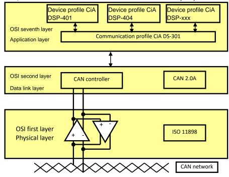
In the OSI model, the relation between the CAN standard and the CANopen protocol is as follows.
