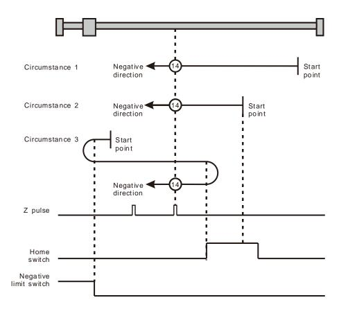
Homing depending on the home switch, negative limit switch and Z pulse ((1): mode 14)
