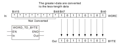
> The Bit-string data are converted into the Bit-string data as the following table shows.
