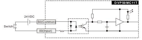
■ The input points of DVP-50MC series motion controller, 10~17 correspond to S1 as shown below.
