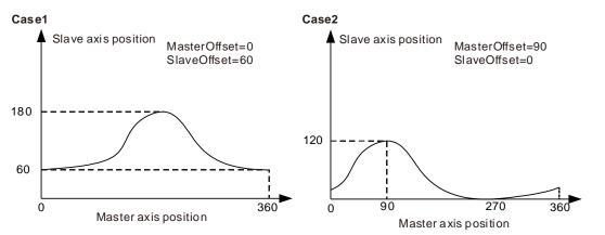
**Case 1.** The slave axis position corresponding to the master axis position will add by 60 based on the planned position as *MasterScaling* and *SlaveScaling* are both 1, *MasterOffset* is 0 and *SlaveOffset* is 60.
