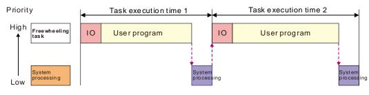
**Note:** There is no fixed execution time for the freewheeling task. So the values of task execution time 1 and task execution time 2 may not be equal in the above figure.
