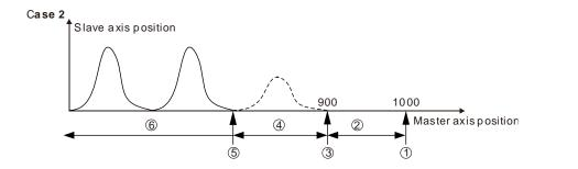
**Stage 1:** Trigger and execute the MC\_CamIn instruction. The master axis absolute position is 1000 at the moment. (The absolute axis phase is 200)
