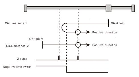
Homing depending on the negative limit switch and Z pulse (①: mode 1)
