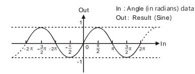
Users can choose different data types for the input parameter in this instruction. But the data type of the output parameter is restricted to LREAL. An error will occur during the compiling of the software if the data type of the output parameter is not LREAL.
