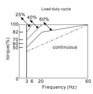
If 100% continuous torque is required at low speed, it may be necessary to use a special inverter duty motor.
