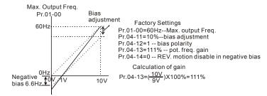
Example 7: Use of 0-10V potentiometer signal to run motor in FWD and REV direction
