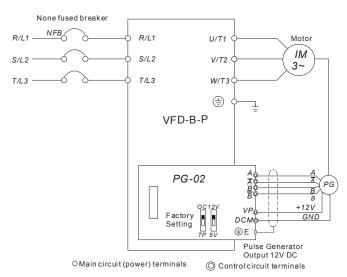
PG-02 and Pulse Generator Connections
