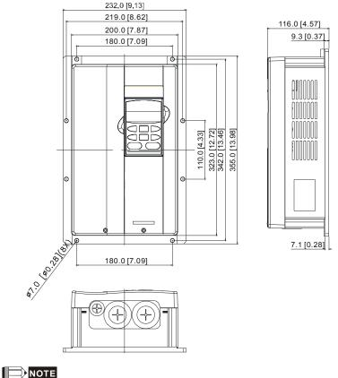
This is only the dimension of the AC motor drive and it needs to be used with a capacity module to be a complete product.
