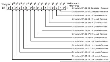
The setting value = bit1 $^{4}$ x2 $^{14}$ +bit13x2 $^{13}$ +....+bit2x2 $^{2}$ +bit1x2 $^{1}$ +bit0x2 $^{0}$  = 1x2 $^{1}$ +1x2 $^{1}$ +1x2
