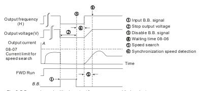
Fig. 2: B.B. speed search with min. output frequency upward timing chart
