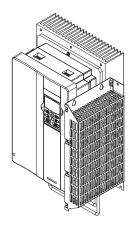
7.5-20HP/5.5-15kW optional heatsink (MKB-PHC1) VFDXXXB43P-C1
