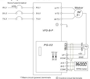
PG-02 and Pulse Generator Connections
