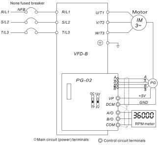
PG-02 and Pulse Generator Connections
