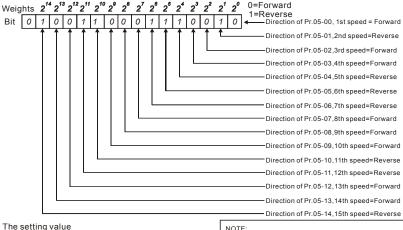
The setting value = bit14x2<sup>14</sup>+bit13x2<sup>13</sup>+...+bit2x2<sup>2</sup>+bit1x2<sup>1</sup>+bit0x2<sup>0</sup> =  $1x2^{14}+1x2^{11}+1x2^{10}+1x2^{5}+1x2^{5}+1x2^{4}+1x2^{1}$ = 16384+2048+1024+64+32+16+2=19570Setting 05-16
