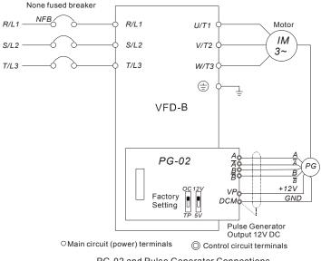
PG-02 and Pulse Generator Connections
