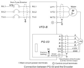
2. Connect Externally with the Encoder of 5V Power Supply and Output Signals to
