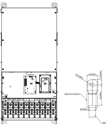
Control Terminal Torque: 4Kgf-cm (3 in-lbf) Wire Gauge: 12-24 AWG
