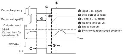
Fig. 2: B.B. speed search with last output frequency downward timing chart
