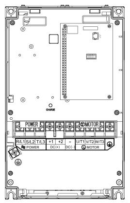
Control Terminal Torque: 4Kgf-cm (3 in-lbf) Wire Gauge: 12-24 AWG (3.3-0.2mm<sup>2</sup>)
