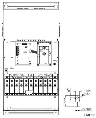
Control Terminal Torque: 4Kgf-cm (3 in-lbf) Wire Gauge: 12-24 AWG
