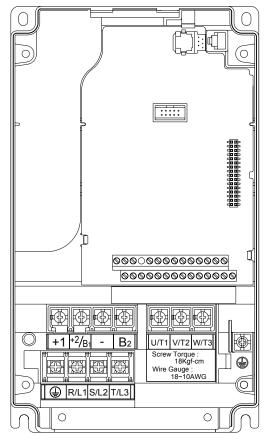
Control Terminal Torque: 4Kgf-cm (3 in-lbf) Wire Gauge: 12-24 AWG(3.3-0.2mm<sup>2</sup>)
