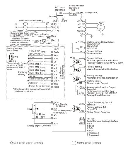
Figure 5 Wiring for SINK mode and SOURCE mode
