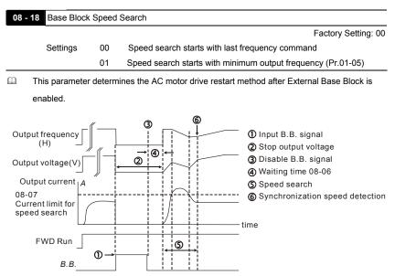
Fig. 1: B.B. speed search with last output frequency downward timing chart
