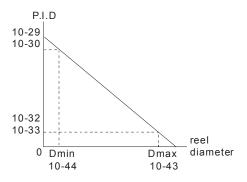
When this parameter is set to 02, two sets of PID parameters are used, where Pr.10-29 ~ 10-31 corresponds to Pr.01-05; Pr.10-32 ~ 10-34 corresponds to Pr.01-00, they are linear.
