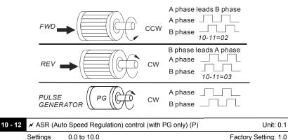
This parameter specifies Proportional control and associated gain (P), and is used for speed
