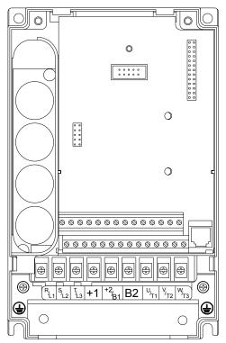
Control Terminal Torque: 4Kgf-cm (3 in-lbf) Wire Gauge: 12-24 AWG(3.3-0.2mm<sup>2</sup>)
